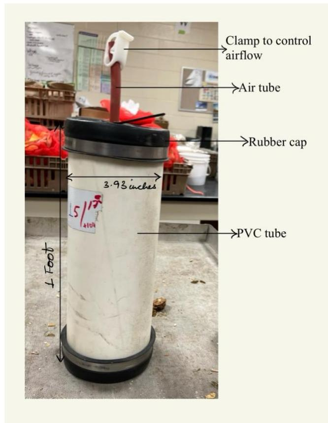
Figure S1. Mini-silo (made from polyvinyl chloride (PVC) pipe) used to study different compaction density.
