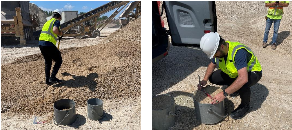
Figure 3.8 Unit box test: (a) filling, (b) leveling
