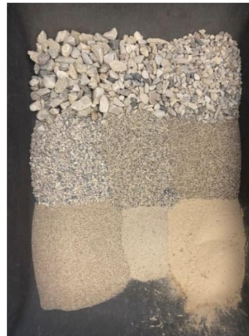
Figure 3.13 Gradation controlled sample preparation
