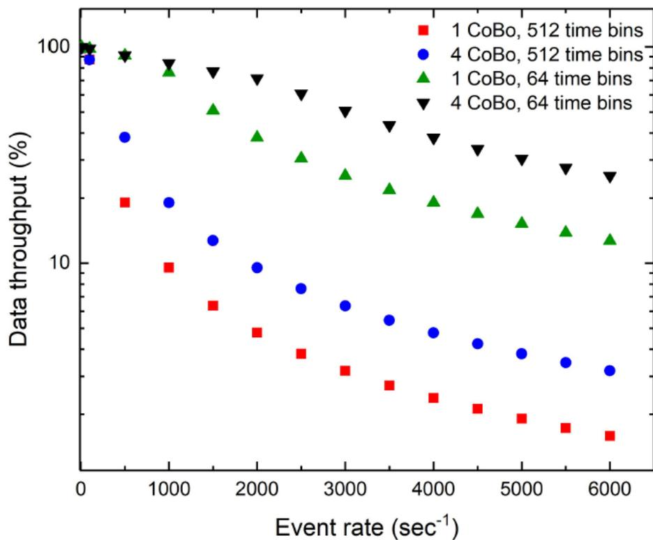
Figure 4.8: Data throughput as a function of event rate for various time binnings and CoBo configurations [31].
