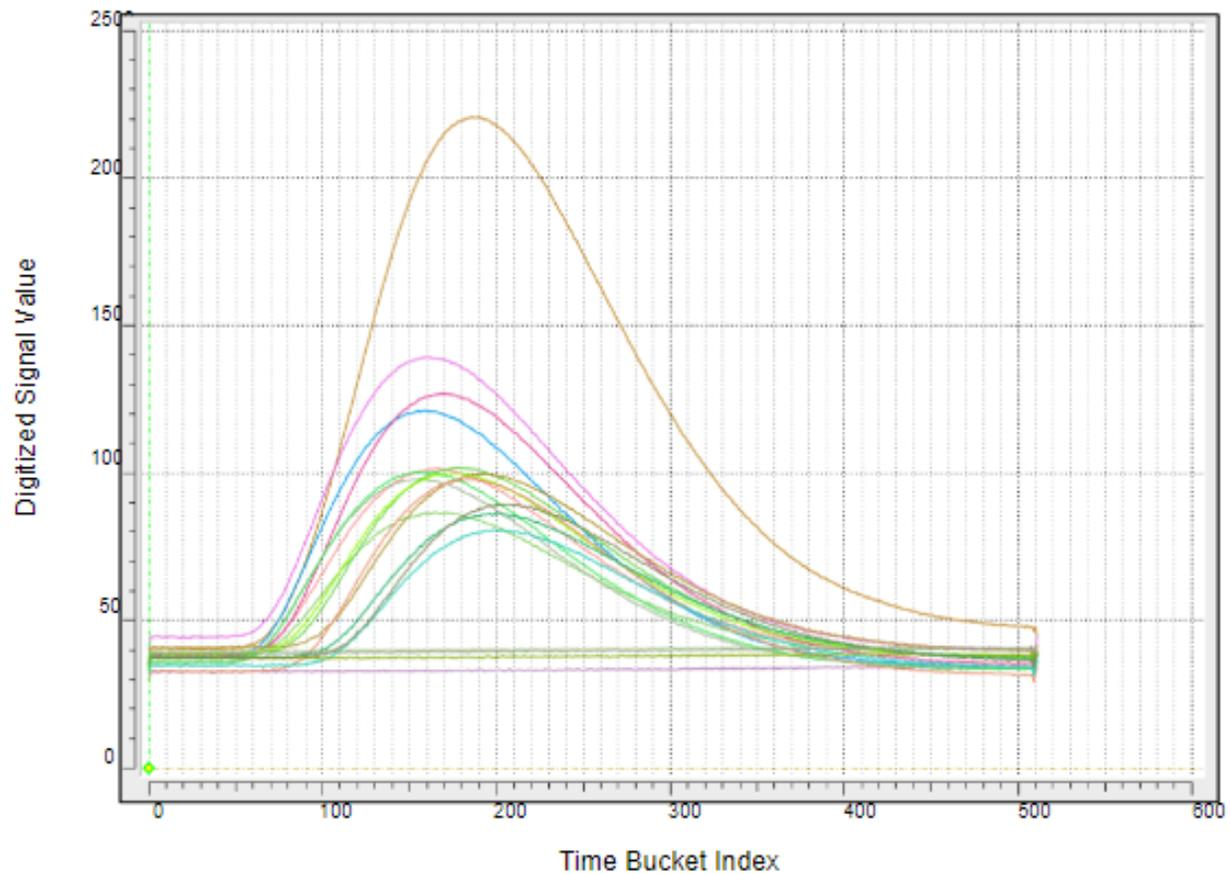
Figure 5.1: Traces on a single AGET chip for a typical TPC event. Each trace represents the signal from one pad. Each trace spans 512, 10 ns time bins and the integral of each trace corresponds to the energy collected.
