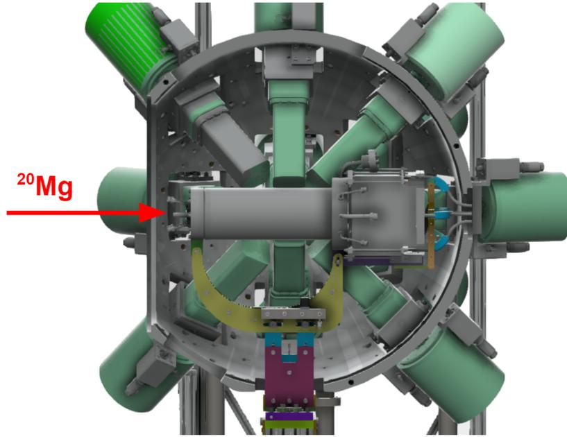
Figure 4.3: Schematic representation of the FRIB Decay Station's DEGAi, featuring the TPC and AsAd box at the core. A red arrow illustrates the entry path of a  $^{20}\text{Mg}$  beam into the TPC, and DEGAi is used to measure gamma-rays emitted from the TPC following nuclear decay.
