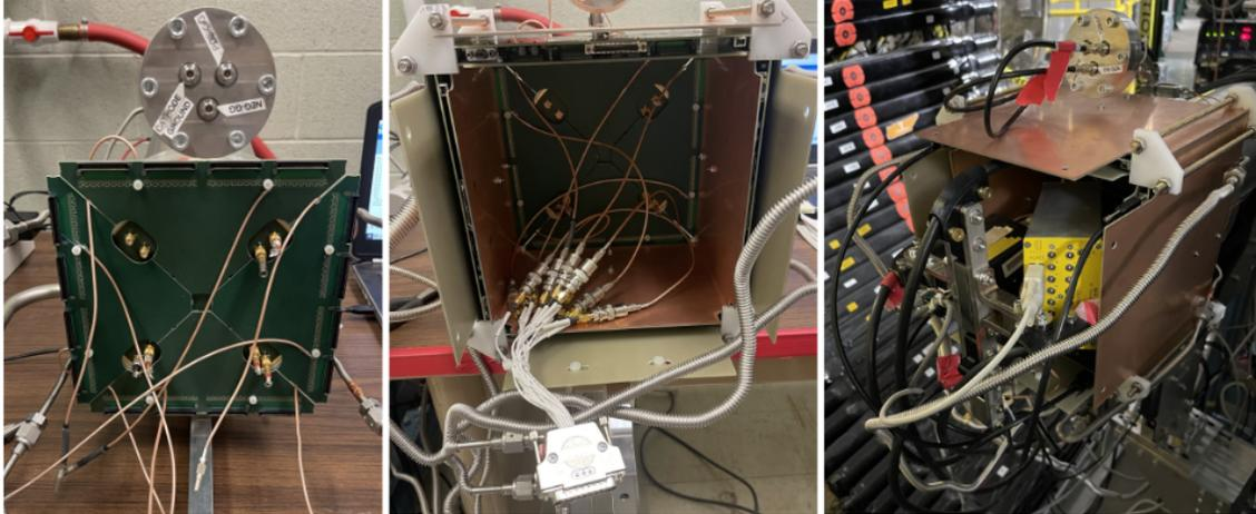
Figure 4.10: Images showing the construction of the front-end veto condition. Left) Image of the soldered lemo connections on the capacitor pads of the zap boards that correspond to each veto pad. Middle) Veto connections integrated into single input for a preamplifier, and AsAd boards are connected with copper shielding. Right) Full AsAd box setup with front-end veto condition fully implemented.
