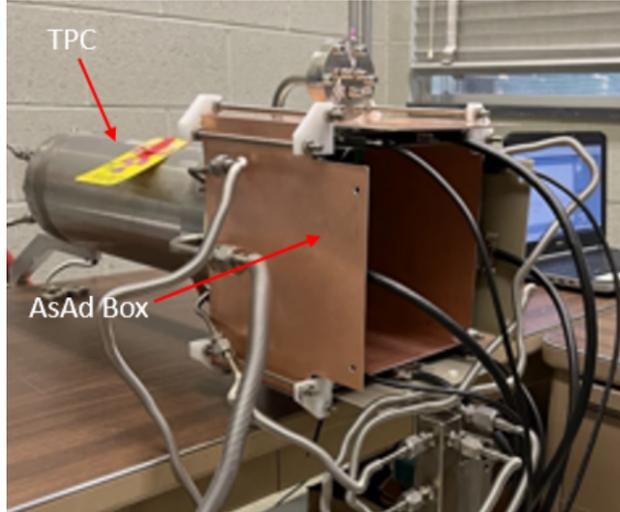
Figure 3.1: The GADGET II TPC in a lab space off the beam line.
