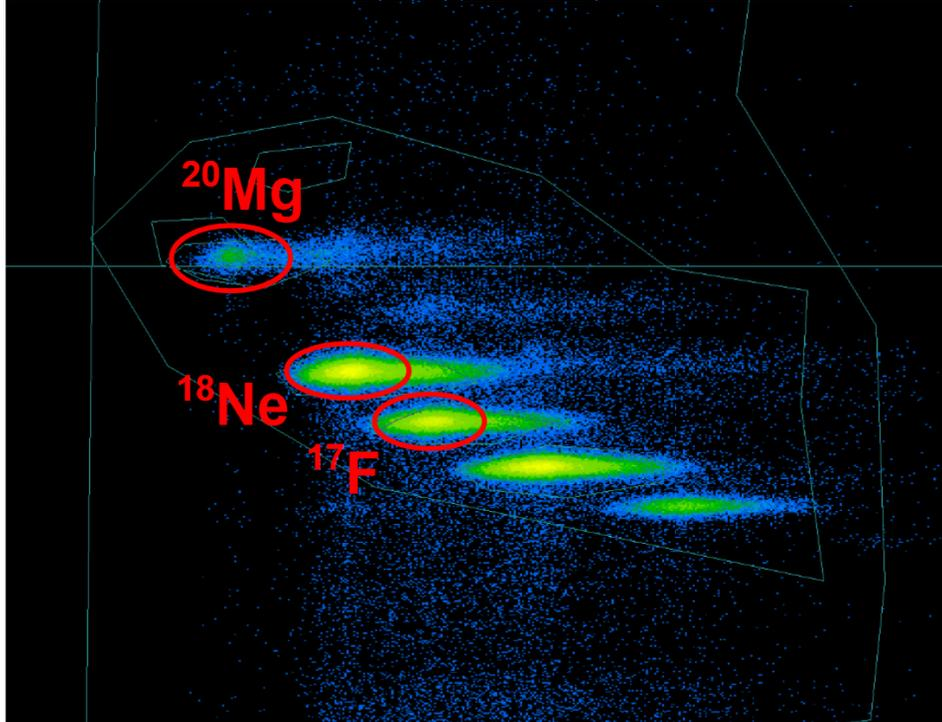
Figure 4.6: PID plot generated using the  $\Delta E$ -TOF technique for precise particle differentiation. The plots shows that  $^{20}\text{Mg}$  was in the beam, along with some other contaminants.
