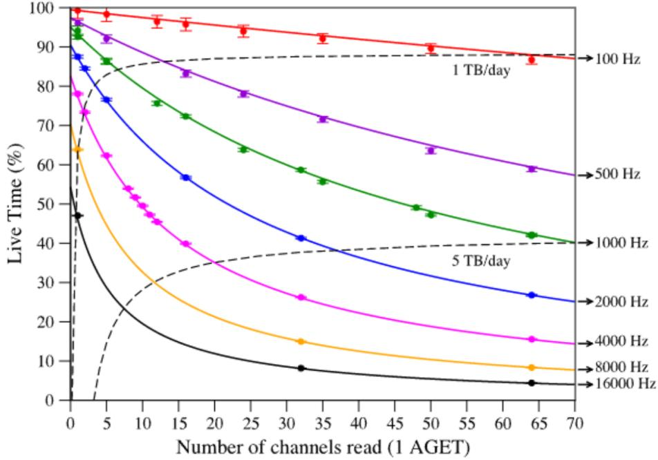
Figure 4.7: Live time of the GET system as a function of channels read for one AGET chip. The plot illustrates the system’s performance degradation with increasing event rates and channel activity.
