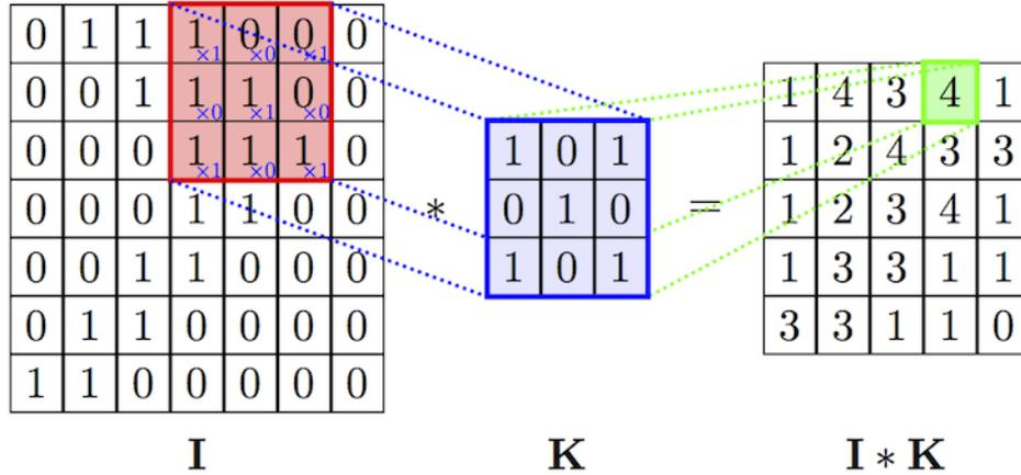
Figure 6.1: An illustration of the convolution process. The input is a 7 x 7 image with a 3 x 3 filter. The output feature map has dimensions 5 x 5 [60].
