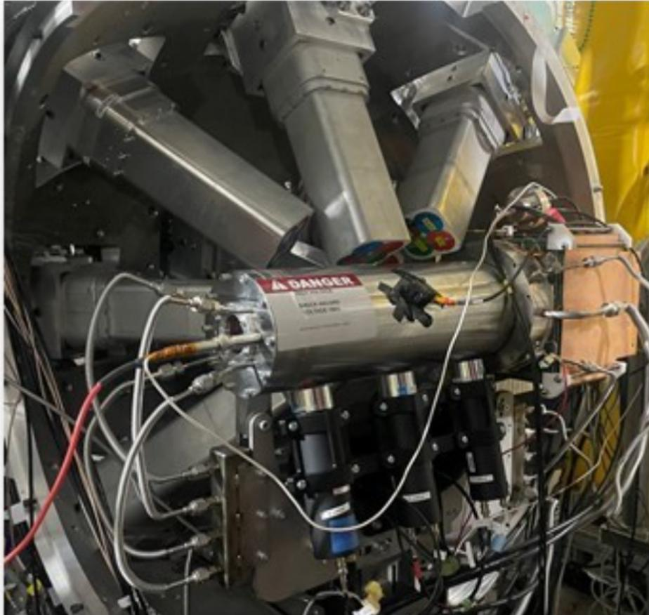
Figure 4.5: Image of the experimental GADGET II setup. The TPC and AsAd box are positioned at the center of the CLARION1 array by a newly built support structure that includes a new gas manifold and three  $\text{LaBr}_3$  detectors. Surrounding the TPC on one side is DEGAi.
