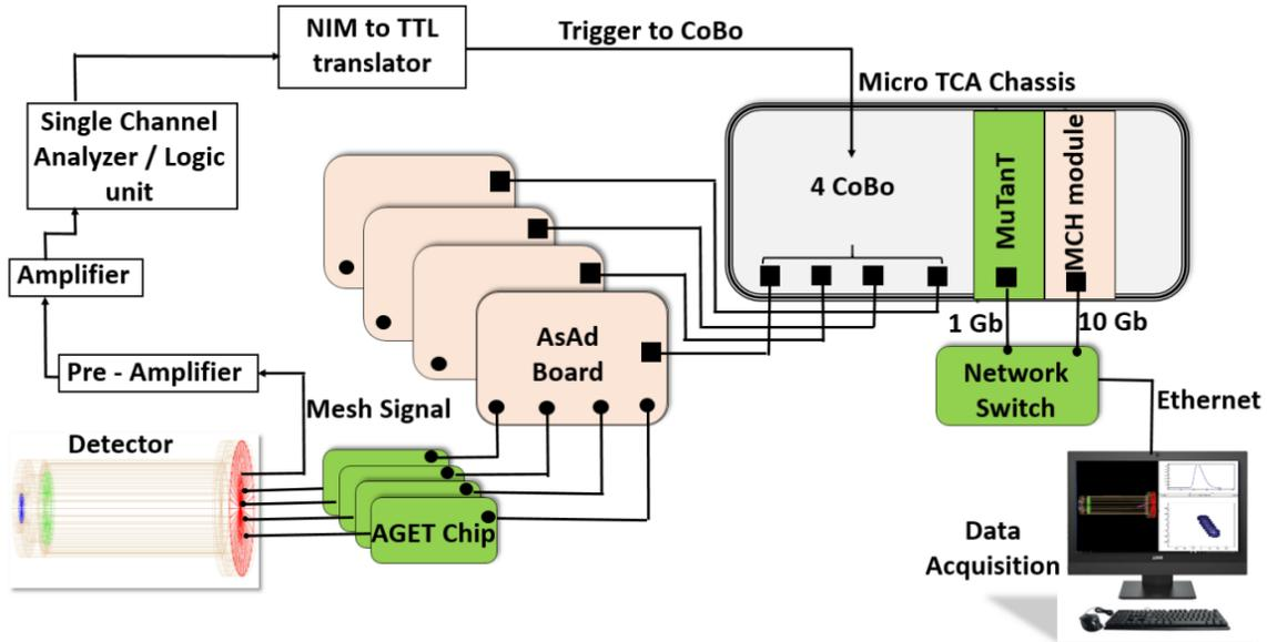
Figure 3.4: Simplified schematic of the GET system with a single  $\mu$ TCA (Micro Telecommunications Computing Architecture) chassis, 4 CoBos (Concentration Board) and a MuTanT (Multiplicity Trigger and Time).
