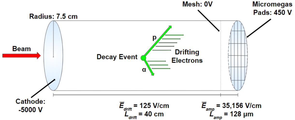
Figure 3.2: Simplified schematic of the GADGET II TPC.
