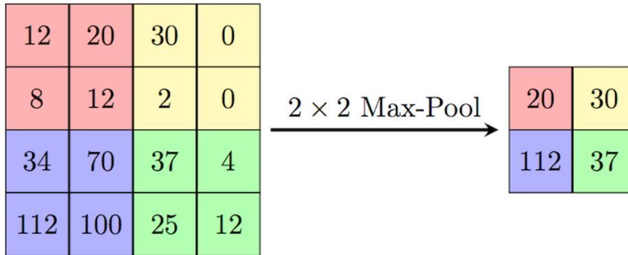
Figure 6.2: Illustration of reducing the dimensions of a feature map using  $2 \times 2$  max pooling [63].
