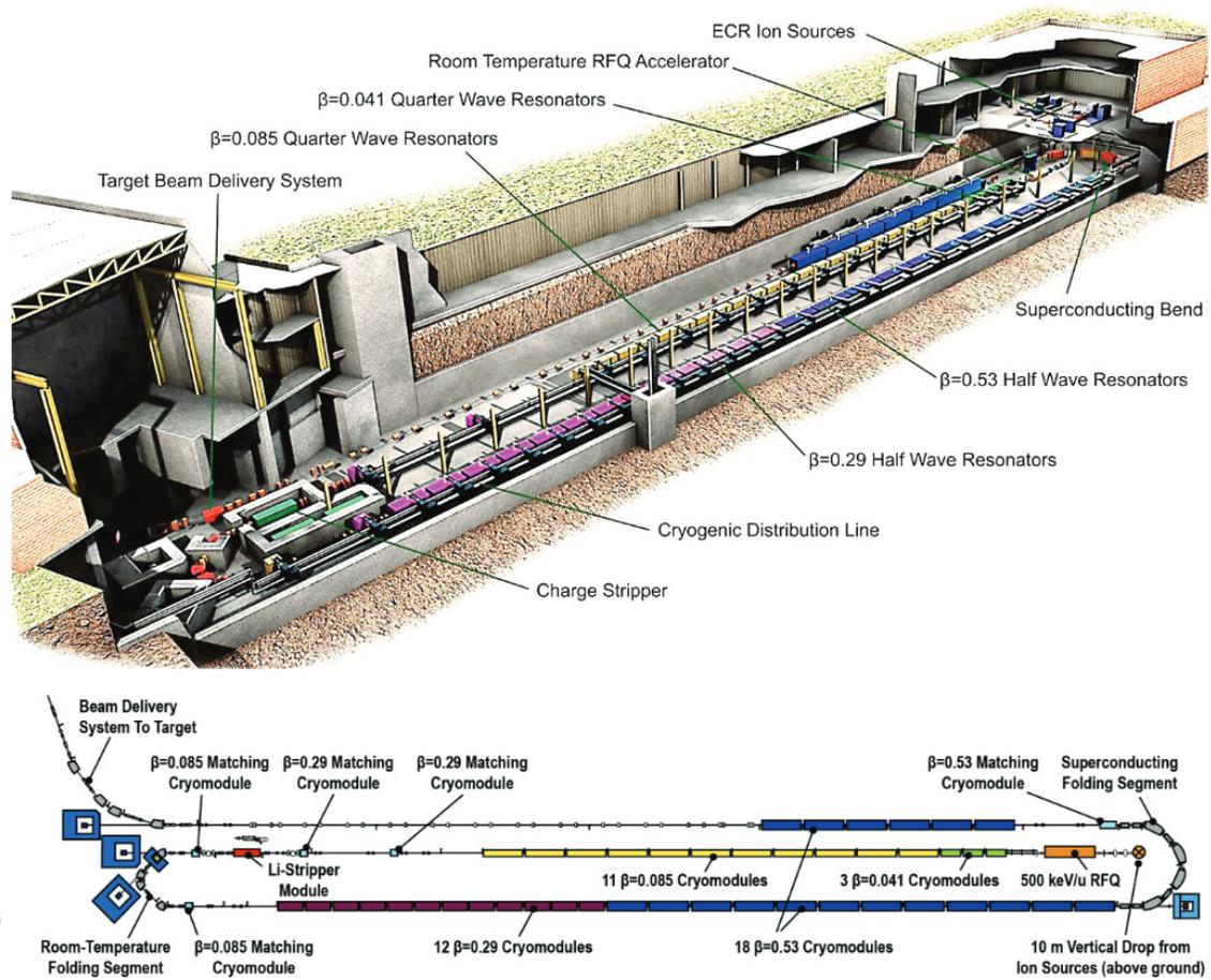
Figure 4.1: Top) Scale 3D rendering of the superconducting radio-frequency driver linear accelerator at FRIB. Bottom) Schematic layout of the FRIB driver linac [50].
