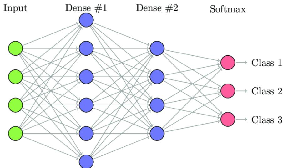
Figure 6.3: Representation of fully connected layers [64]. The input, after being flattened, passes through 3 FC layers. The final layer utilizes a softmax activation function to yield probabilities for each class.
