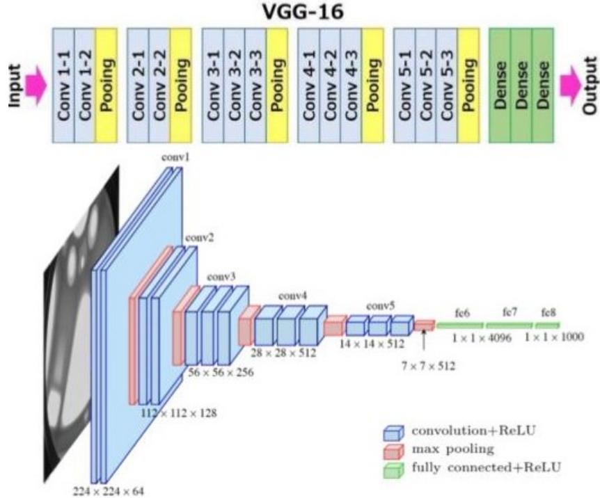
Figure 6.4: A depiction of the VGG16 architecture, illustrating the orderly sequence of layers from the initial input to the final output [65]. The upper segment of the Figure elucidates the journey from the raw input through a series of convolutional and pooling layers. The lower segment visualizes the transformation of an input image as it traverses through the network, delineating the evolution in dimensions and depth of the feature maps at various junctures.
