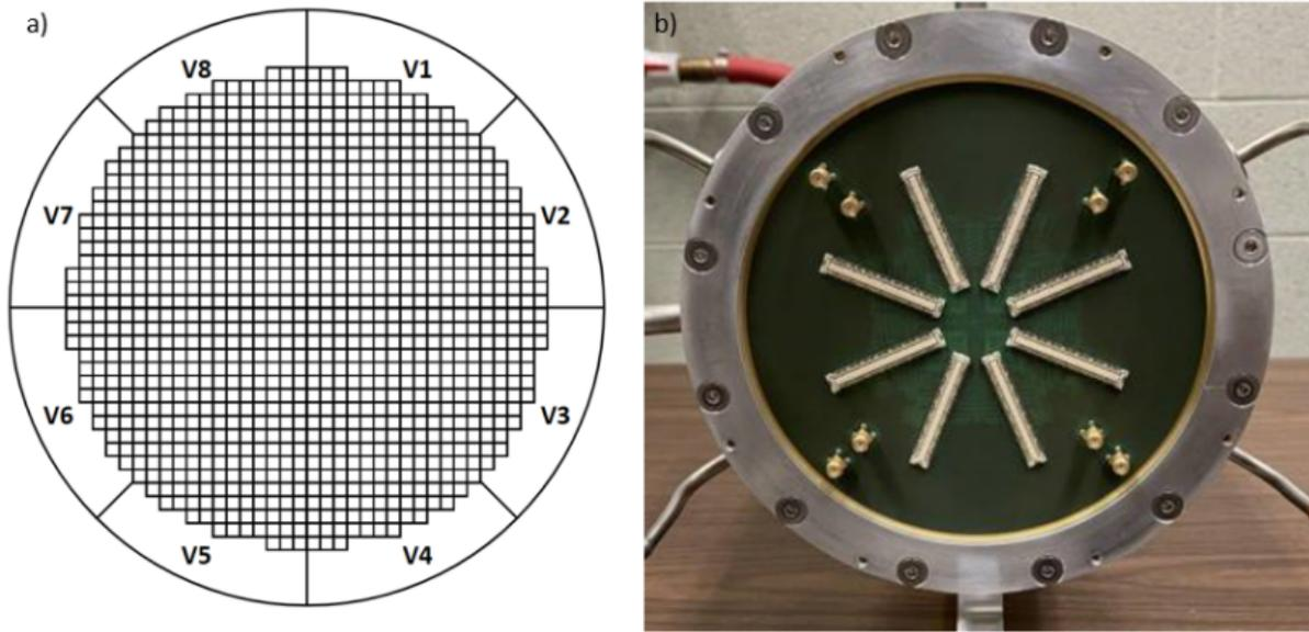
Figure 3.3: a) Schematic of the MM board's front view, illustrating the central region composed of 1016 measurement pads, along with 8 veto pads labeled V1 to V8. b) A view of the MM board's rear end cap, showing 8 multi-pin connectors, each with 144 channels, which are then connected to the T-Zap boards (not depicted).
