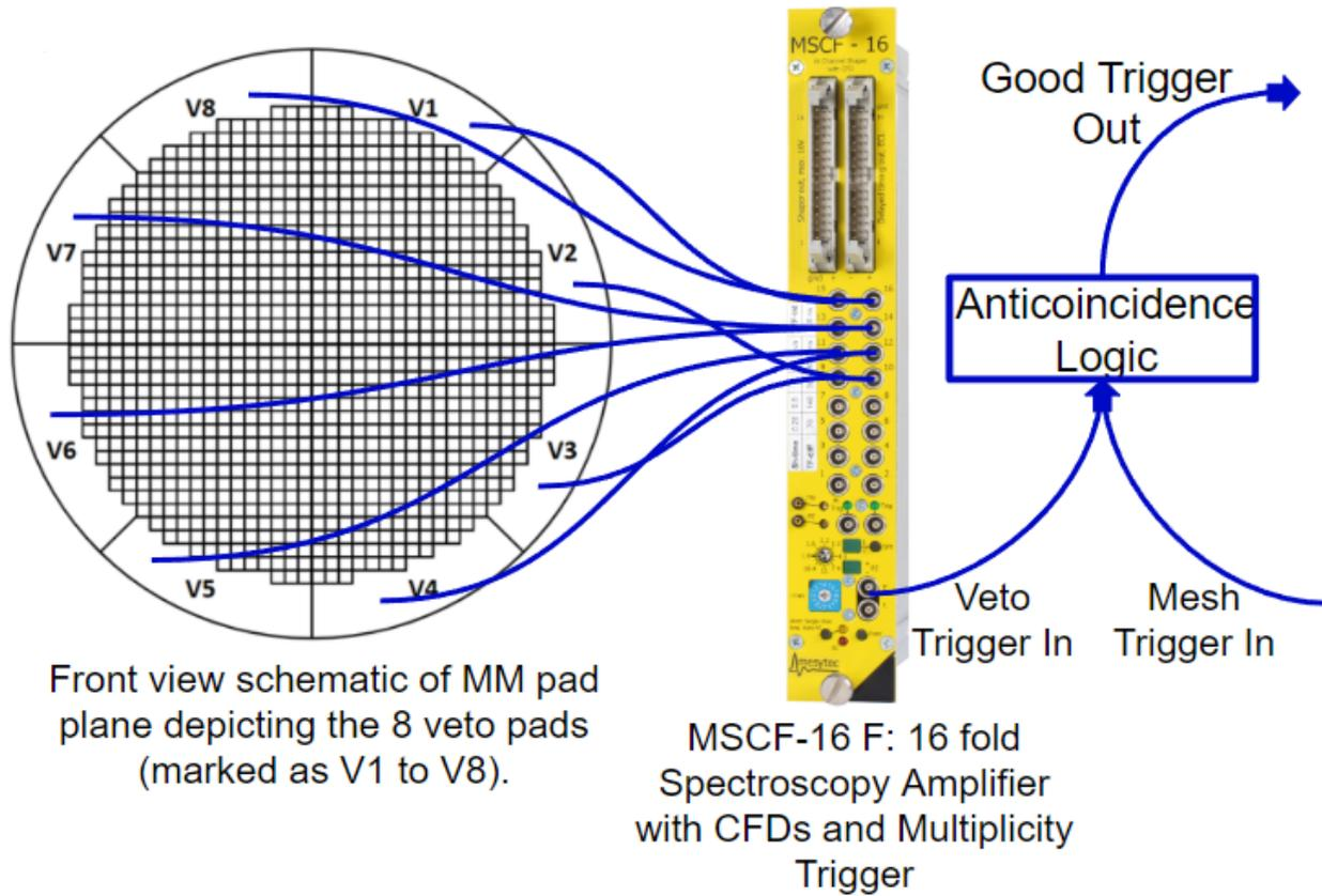
Figure 4.9: Schematic diagram of the front-end trigger veto condition showing the pad plane, connections to the veto pads (marked V1-V8), and the module used to create an output trigger if any signal arrives at the veto pads. The output trigger from the MSCF-16 F module is then placed in anticoincidence with the mesh event trigger.
