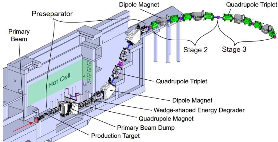
Figure 4.2: This ARIS diagram illustrates the driver linac’s primary beam approaching the production target from the lower left. Isotope beams travel through the three stages of the fragment separator (preseparator, stage 2, and stage 3) before being channeled towards experimental setups [49].
