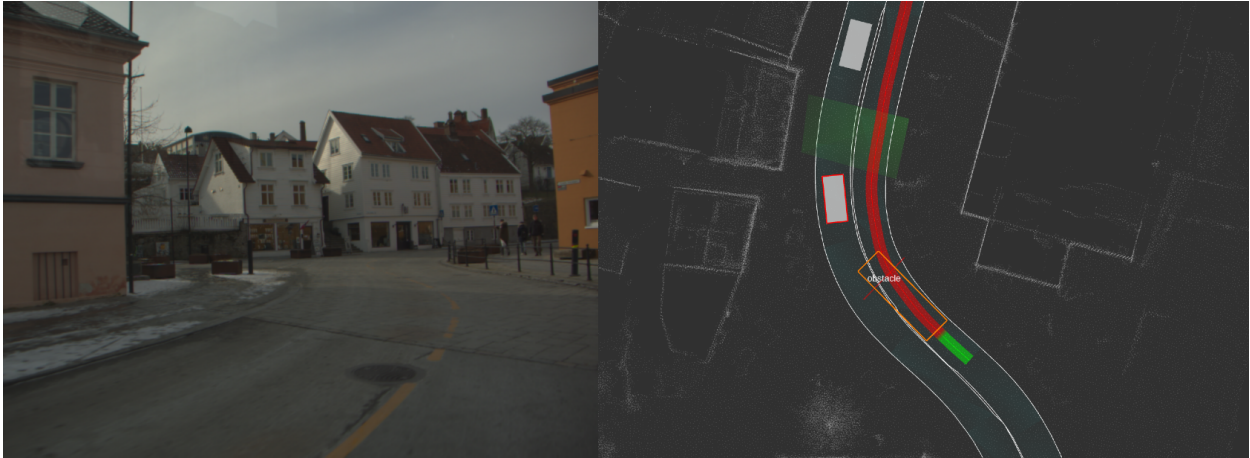
Figure 1.1 A part of the daily route taken by the bus running ADASTEC's software at the city of Stavanger, Norway. On the left is a camera snapshot of the general area, and on the right is the lane excursion scenario replicated in a simulation environment using collected sensor data.
