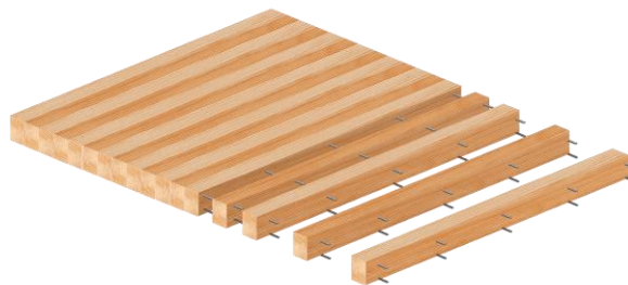
Figure 2.6: Nail Laminated Timber
