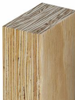
Figure 2.8: Laminated Veneer Lumber
