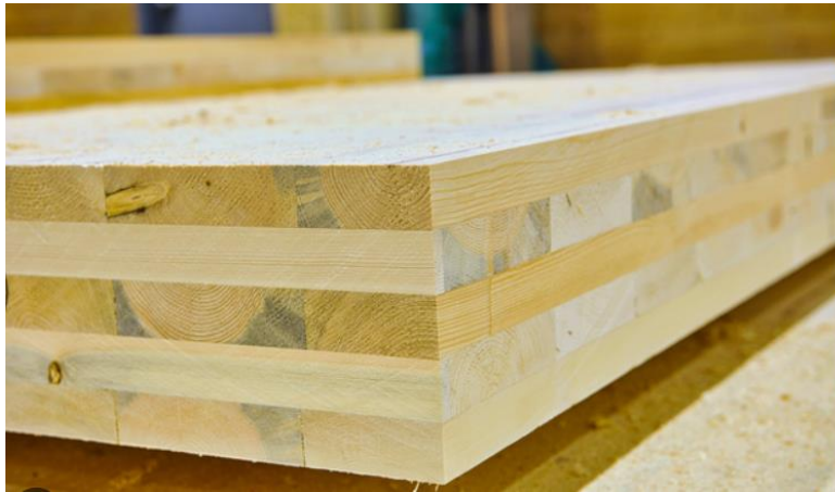
Figure 1.3: Cross Laminated Timber
