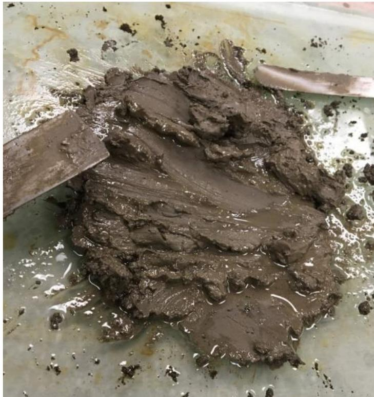
**Figure 3. 1. 1 Leakage of PCM-B during Liquid Limit Test**
