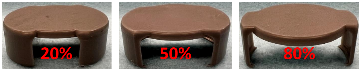
Figure 7. Three variations of outer cap showing the varying size of cutaways. Varying amount of functional surface area of the inner cap available to be gripped and a torque applied to.
