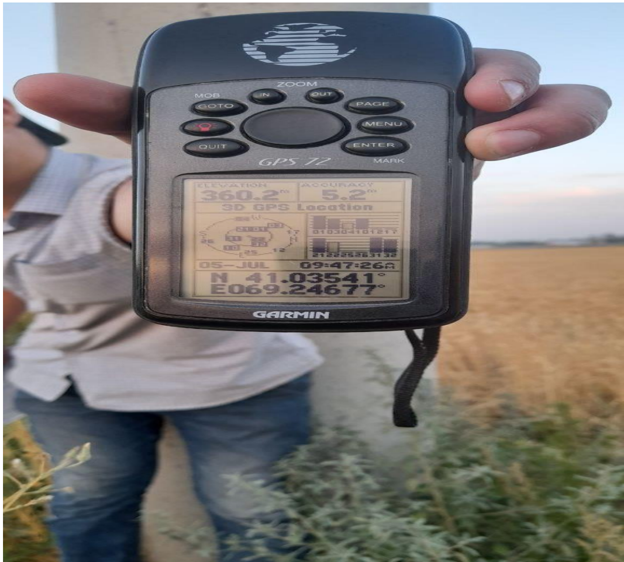
Figure 11. Use of Garmin GPS 72 device in the field for location measurements.
