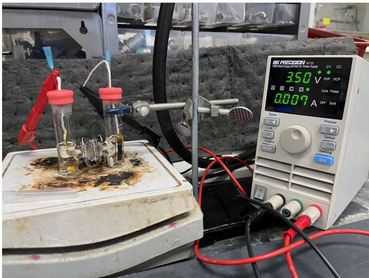
Figure 4.S1. Bulk Electrolysis setup.
