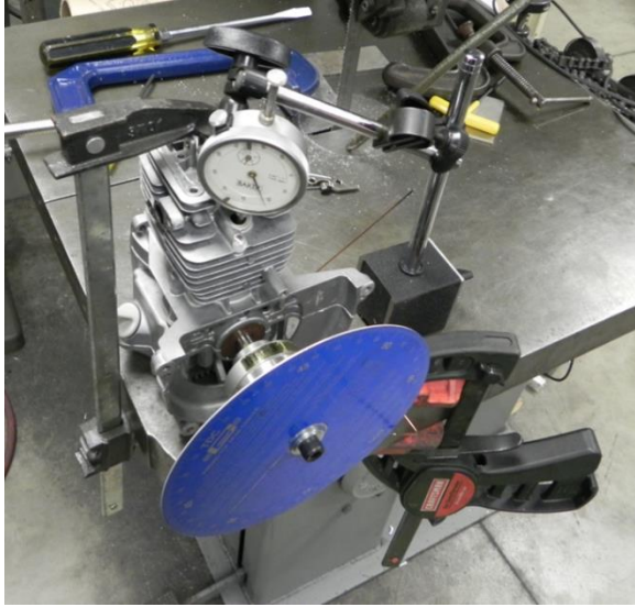
Figure 6. The setup for measuring pushrod displacement with the dial gage positioned to measure TDC
