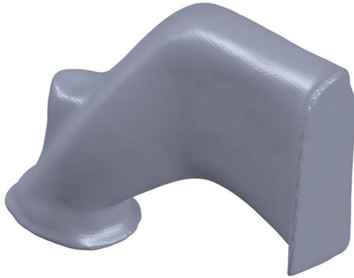
Figure 9-11 Scan results of the positive body casting of the intake port made from the sample cylinder head pictured in Figure 9-1
