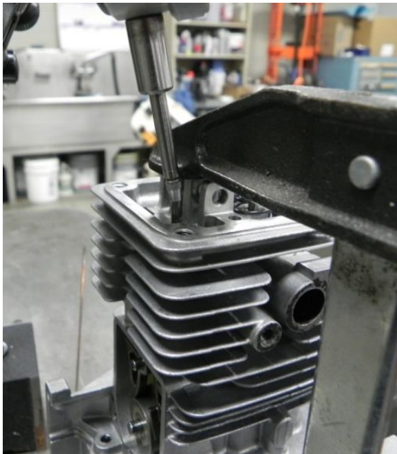
Figure 7. An up close picture showing the dial gage resting on the top of the engine's pushrod
