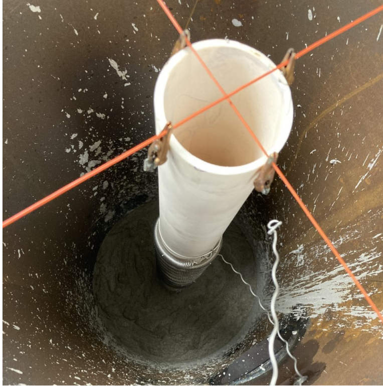
Figure 3.8 The centering process for the alumina reactor tube within the steel shell.
