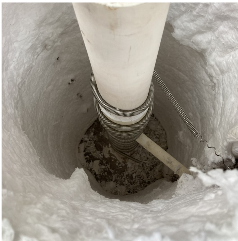
Figure 3.10 Layers of ceramic insulation surrounding the reactor tube. When the reactor is sealed, insulation fills the entire cavity shown in the image.
