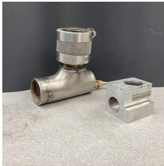
Figure 3.3 The two L-valves utilized by the oxidation reactor, with the earliest design on the right and the latest iteration on the left. The right-angle junction of each valve allows the particle column to pause in between bursts of air.
