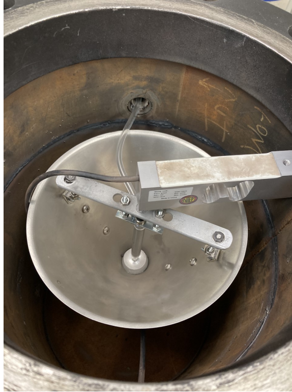
Figure 3.4 The particle "catchcan," consisting of a plugged funnel suspended from a load cell. When full, the plug is removed via a pneumatic piston to allow particles to drain.
