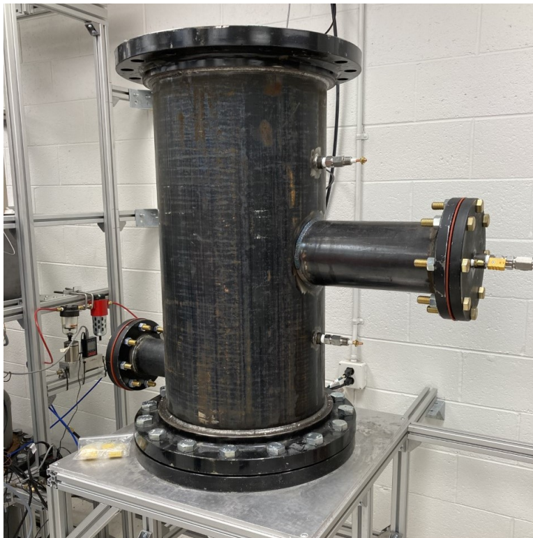
Figure 3.9 The outermost steel shell of the reactor. The tube lies at the center of the shell and is surrounded by fibrous insulation.
