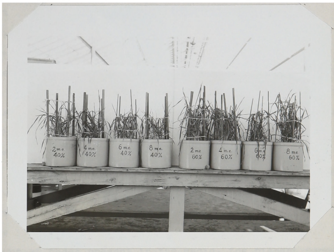
Fig. XII. Rye crops at the end of two months showing no significant difference of the growth by varying the base exchange capacity of the bentonite-sand mixture.
