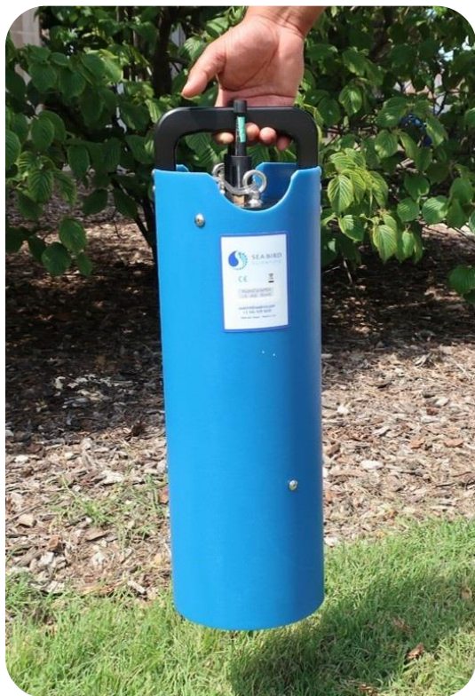
Figure A1.1. Two photos of HydroCycle-PO 4 , with and without shield (Right Image: courtesy of seabird.com).
