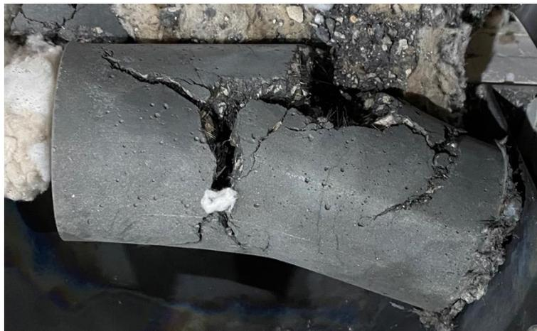
Figure 3.13: Explosive spalling of a large UHPC cylindrical specimen (UHPC-ST-8)
