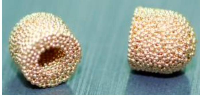
Figure 3.2: Sintered metal heads used in pore pressure measurements [66]
