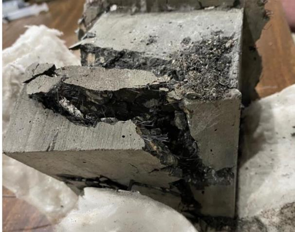
Figure 3.11: Cracking and spalling of UHPC specimens after testing
