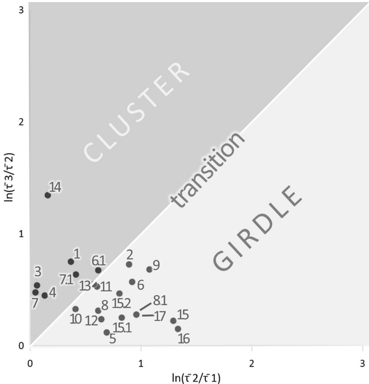
Figure 35. Woodcock Plot (Woodcock, 1977) showing clast macrofabric shape. Data are shown as two-axis logarithmic plot of ratios of normalized eigenvalues \tau_3 , \tau_2 , \tau_1 . Individual data points are labeled. The transition line, labeled, indicates the region in eigenvalue space where clast fabrics above and below the transition line represent cluster or girdle shapes, respectively. The distance from the graph origin is directly proportional to fabric strength; uniform distributions plot at the graph origin whereas progressively stronger preferred clast orientations plot further from the origin (Woodcock, 1977).
