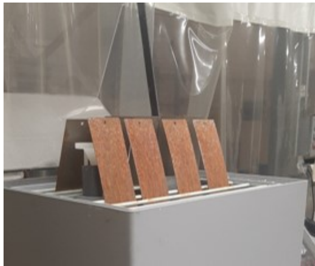
Figure 7.4 Corroded samples inside the salt spray chamber before the 7th day of corrosion.
