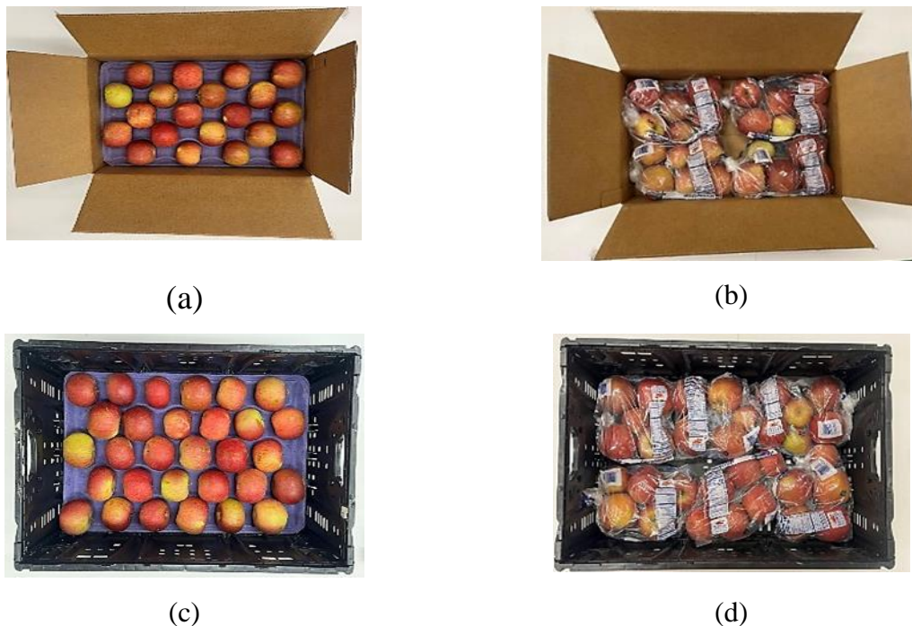
Figure 3.1 package type. (a) RSC + molded paper pulp tray; (b) RSC + plastic bag; (c) RPC+ molded paper pulp tray; (d) RPC+ plastic bag
