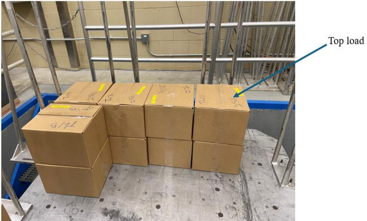
Figure 4.1. Experimental test setup using a vertical vibration shaker table. The top packages with two different weights serve as the top loads
