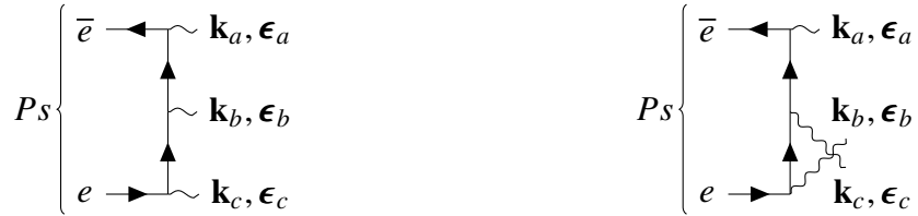
Figure B.1 Two of the six Feynman diagram for 3- \gamma decay of ortho-positronium in QED. The other 4 are generated by cyclic permutation of which photon couples to which vertex.
