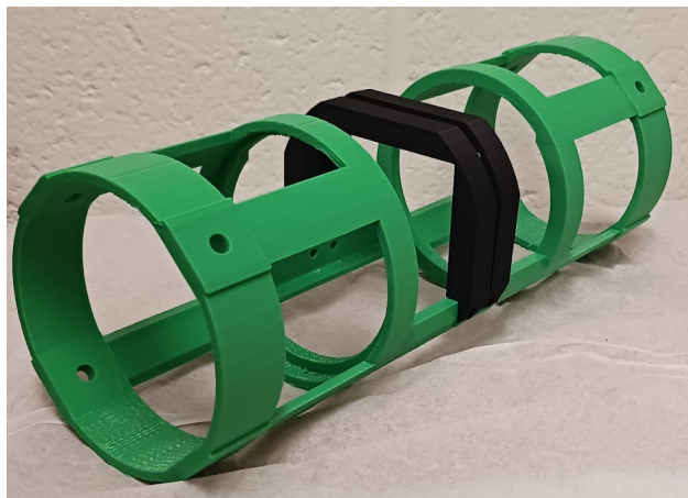
Figure 8.6 Prototype design for the inner module support structure for initial tests in the magnet. This will hold the powder and start detectors centered in the detector array.
