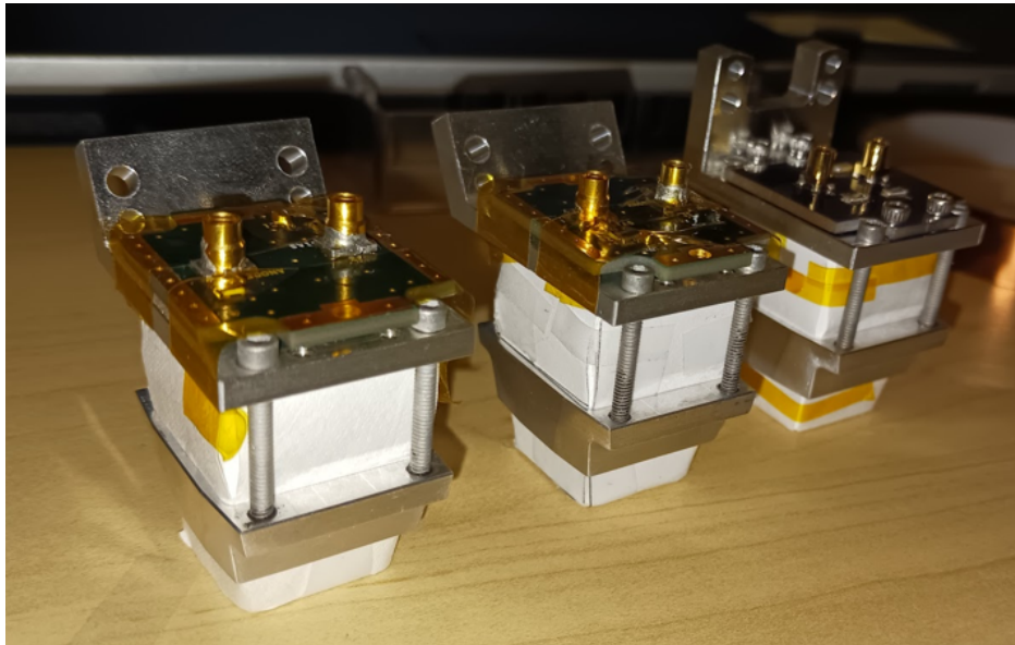
Figure 4.18 Three finalized \gamma -detectors in their clamps. Two of these are with prototype SiPM boards, and one had the finalized board (with the proper screw placement to attach the board onto the back of the crystal).
