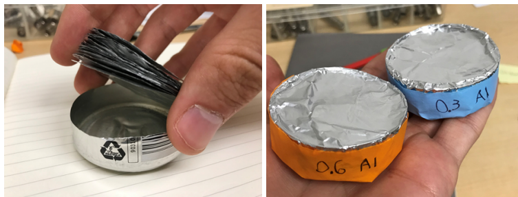
Figure 5.5 Constructed aluminum target designed to match the target densities of the powders to be tested.
