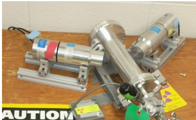
Figure 5.2 Positronium test stand. A vacuum tube connected to a roughing pump, with two \text{LaBr}_3 detectors aimed at a central source in the tube.
