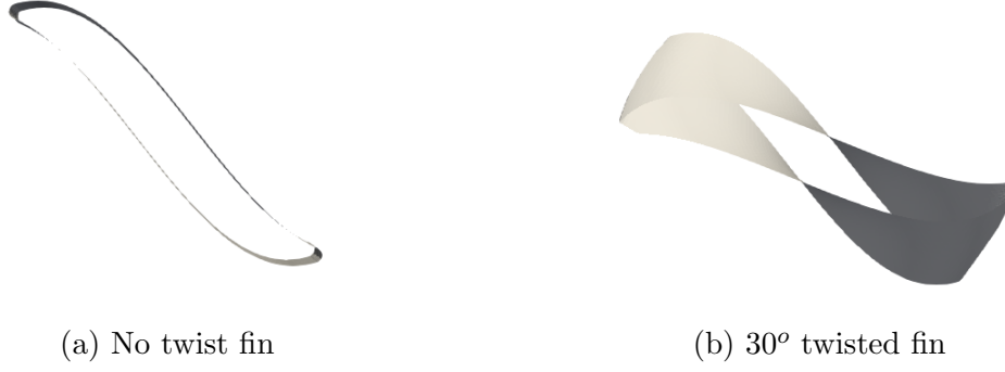
Figure 4.3: 3D twisted S-shaped fins
