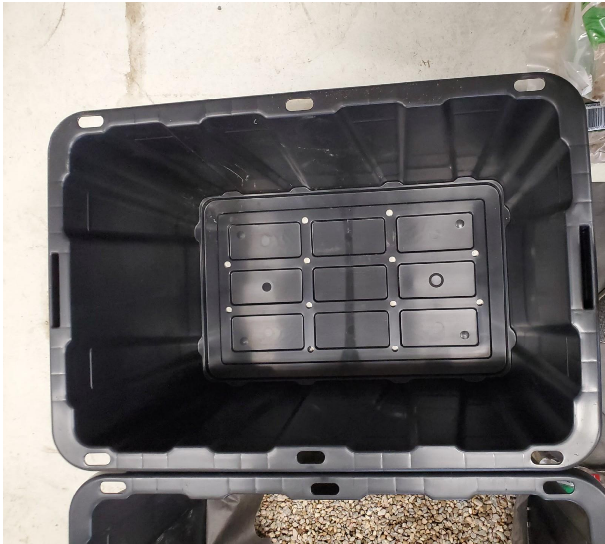
Figure 2. Soil chamber with drainage holes.
