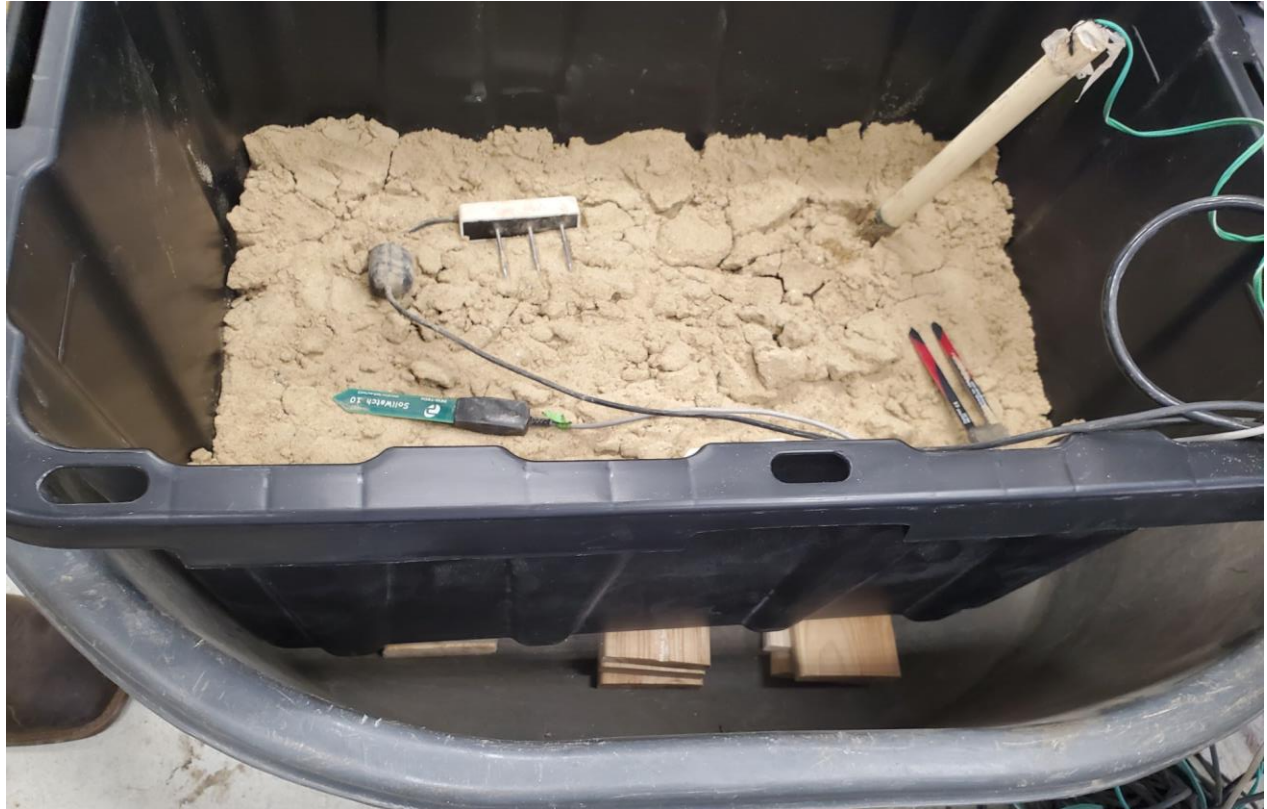
Figure 4. Layout of sensor installation.
