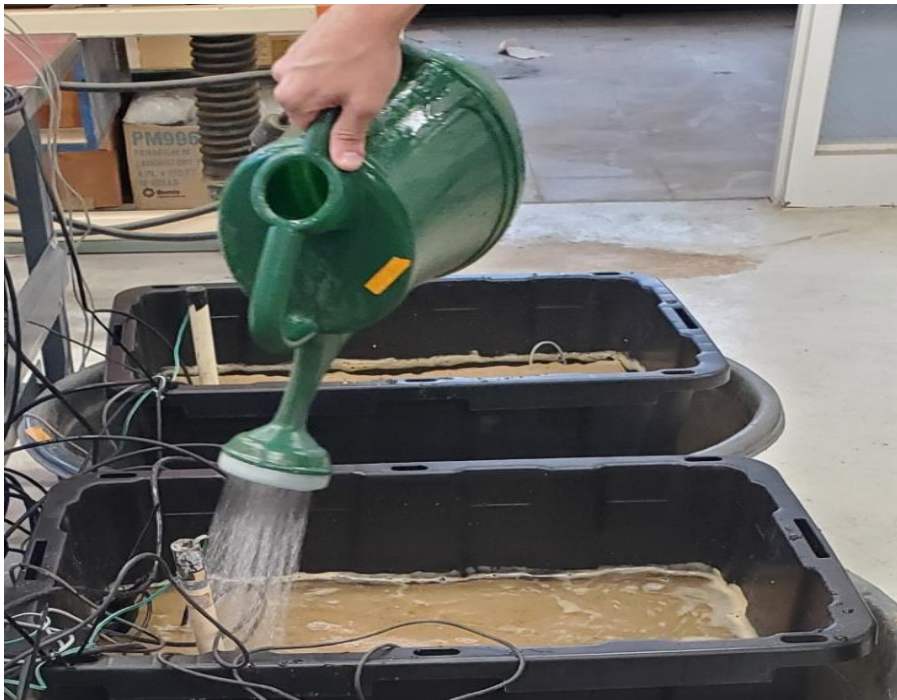
Figure 3. Initial surface irrigation of soil chambers.
