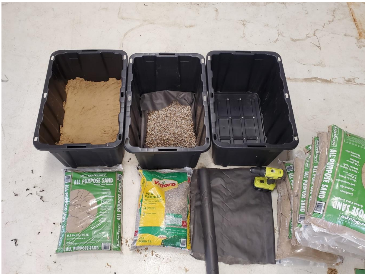
Figure 1. Soil chamber components and construction.
