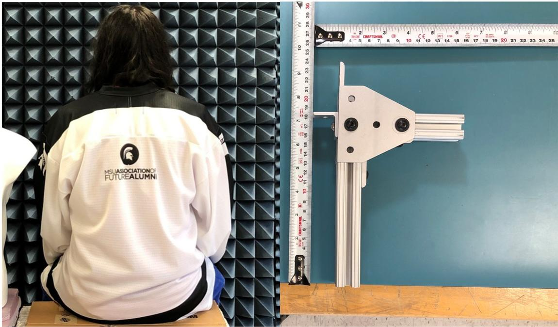
Figure 4.12 **Left:** The subject for the imageless contraband detection experiment which is a real person. **Right:** The object for the imageless contraband detection experiment which is a metallic gun-shape with a dimension of 164 mm×235 mm. Originally submitted to *IEEE Access*, April 2024.
