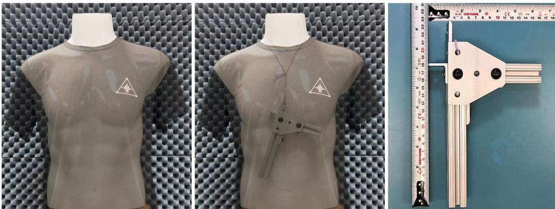
Figure 4.2 From left to right: Front of a clothed mannequin (t-shirt shown transparent to show mannequin); front of a clothed mannequin with a concealed gun-shaped target; the gun-shaped target of dimension 164 mm×235 mm. Image [94] © 2023 IEEE.
