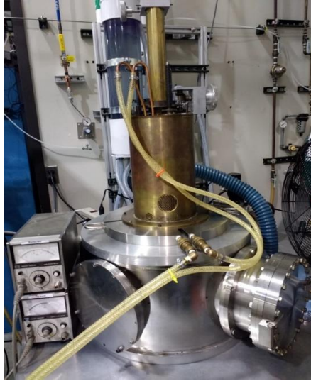
Figure 4.3. Diamond System 6 (DS6) MPACVD reactor for lightly boron doped diamond growth.
