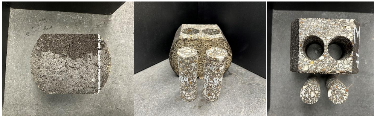
Figure 6-4 Small sample preparation from gyratory pucks used in dielectric-air void calibration
