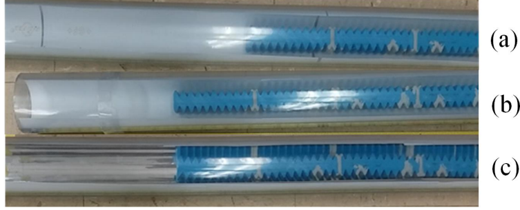
Figure 2.23 Different inner surfaces of pipeline used in the experiments: (a) \mu = 0.53 ; (b) \mu = 1.10 ; (c) \mu = 1.49 .
