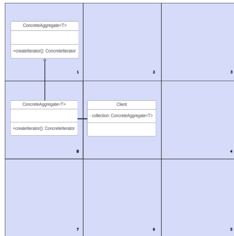
Figure 4.2 Sample layout of a diagram using our testbed. Client was the chosen class and therefore occupies the central cell. Classes with relationships to this class are placed in the cells around the chosen class.
