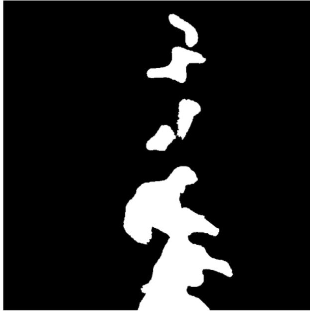
**Figure 2.13:** Processed image of methane flame at the tip section with a Reynolds number of 10000
