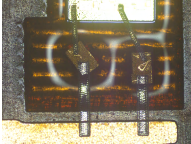
Figure 3.10 An example of the printed die attach method being used to mount SLCs in the same die pocket as the MPA die.
