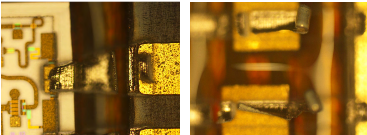
Figure A.6 Printed silver line peeling effect caused by mixing nanoparticle ink with reactive ink.
