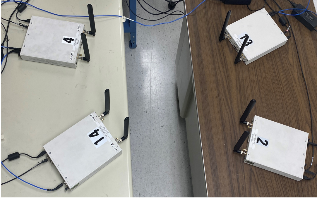
Figure 3.4 Experimental setup composed of four SDRs, with omnidirectional antennas, connected to a single computing unit. The system was designed to wirelessly synthesize two-tone signals without node synchronization. A coarse synchronization is achieved by connecting the SDRs to the same computer and daisy-chaining a reference clock.
