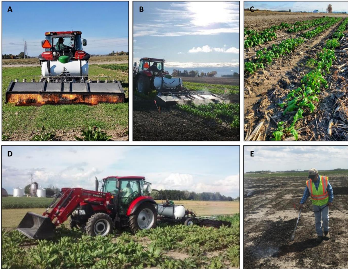
Figure A2.1. (A-B, D) Custom designed 3.25-m wide propane-fueled, tractor-mounted shield burner (Multi-Trail Enterprises LLC) used for application of the fall heat treatments calibrated to heat foliage to 649-871°C. (C) Sugarbeet foliage immediately following 1.6 kmph heat treatment. (E) Handheld Flame King Heavy Duty Propane Torch Weed Burner (Pico Rivera CA 90660) used to apply spring heat treatments.
