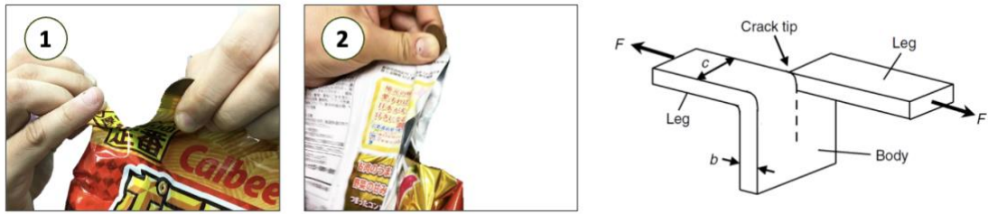
Figure 30 Opening mechanism with Pre-cut Notch (McGee, 2017; Andreasson & Kao-Walter, 2013)
