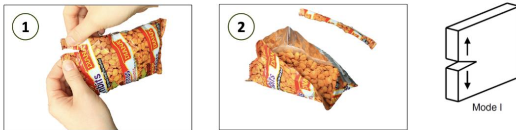
Figure 32 Opening Technique: Side Bowl Tear with Mode I (In-Plane Opening)
