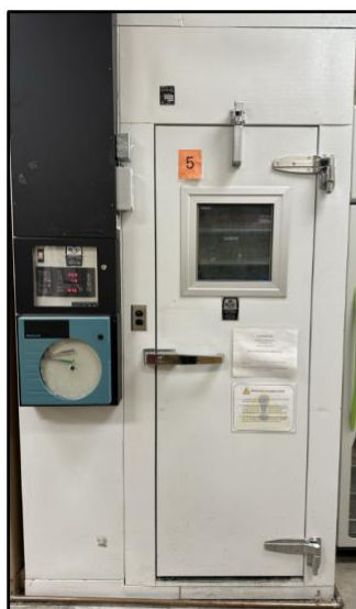
Figure 41 Environmental Growth Chamber set at Room Conditions settings (School of Packaging, MSU)
