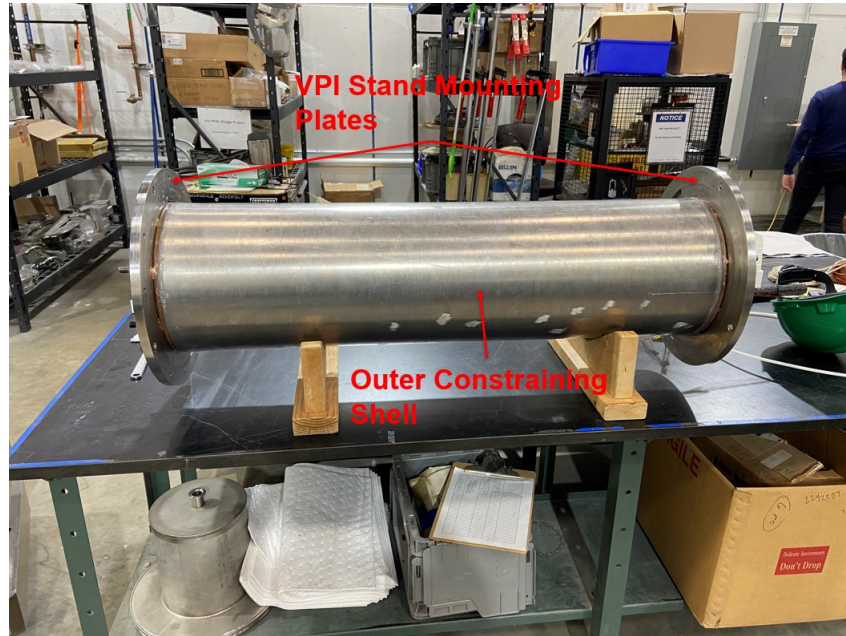
Figure 4.18 Picture of CDQ single layer coil fully prepared for vacuum impregnation process [29].
