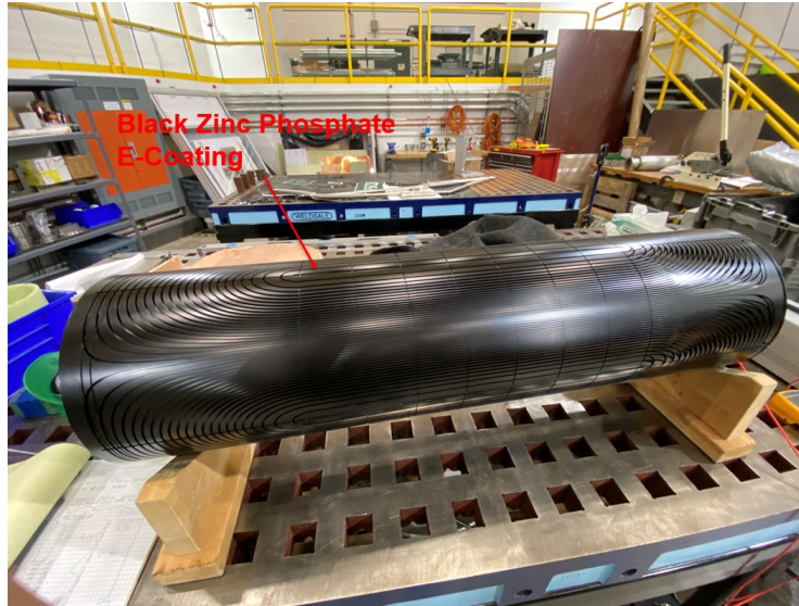
Figure 4.7 Winding bobbin after electro deposition of zinc phosphate "e-coating" completion, the bobbin is then placed on the winding table for real winding of quadrupole.
