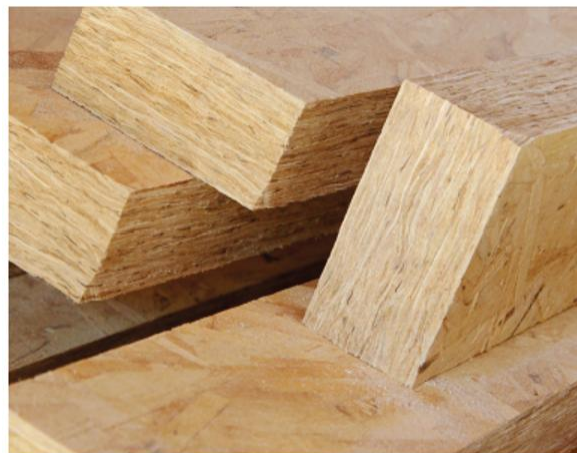
Figure 5 LSL beams (Woodworks 2021)
