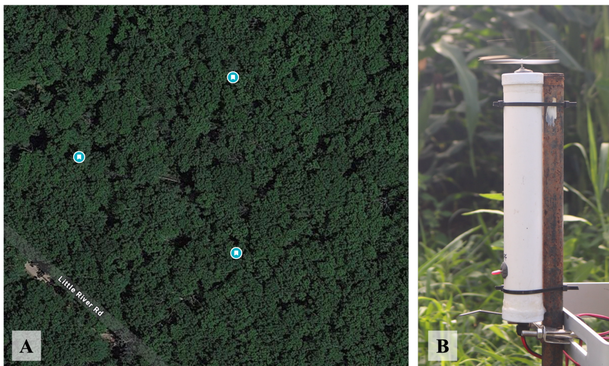
Figure 4.3. Representative photos of field site set-up. A) Topographical map of the equilateral triangle formation of spore traps at each site. B) An example rotating-arm spore trap.
