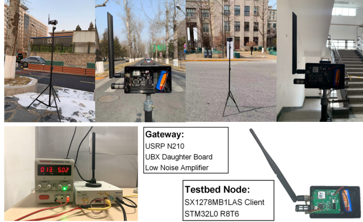
Figure 6.11 USRP N210 based gateway and COTS LoRa nodes deployed in a campus environment.
