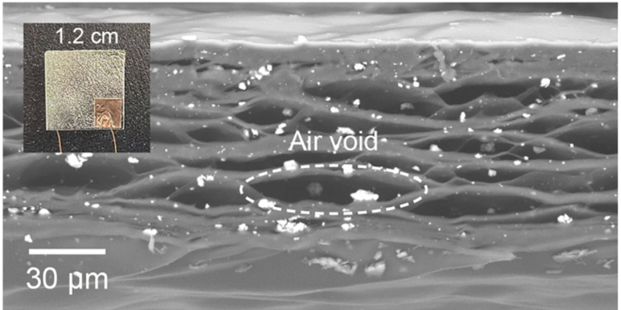
Figure 2.3 SEM image of the cross-sectional view of a PP-based ferroelectret device. The inset shows a PPFE sensor. Reproduced with permission from [30] © 2022 IEEE.
