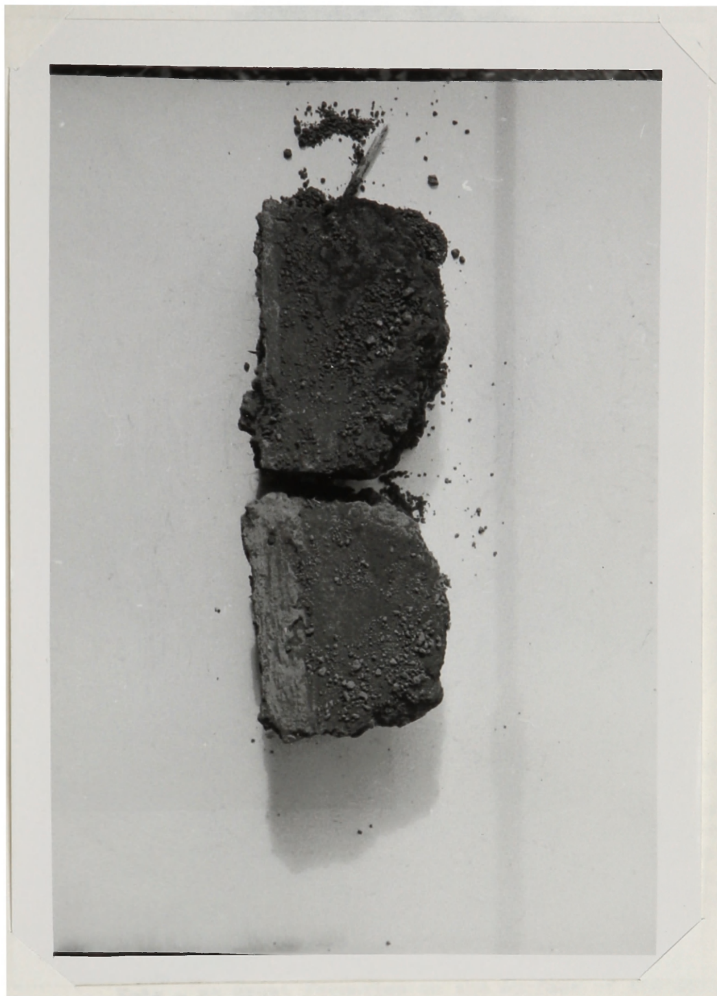
Plate 2. The effect of two crop rotations upon crust formation of soils subject to a (left) cash crop rotation (Rot. 6) and to a legume rotation (Rot. 7). Samples for this picture were taken from the core plots in August, (compare with plate 8)
