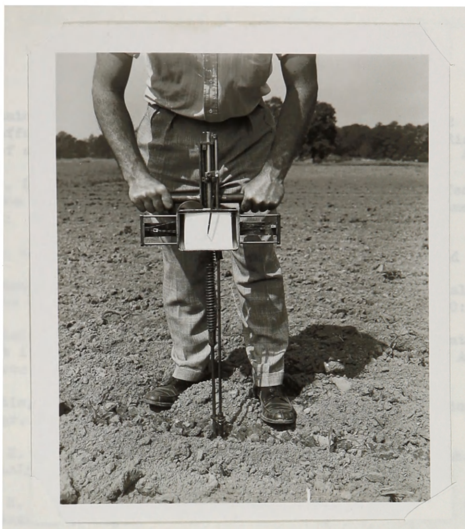
Plate 9. Soil penetrometer developed to measure relative soil conditions. A probe is slowly forced into the soil and a curve is drawn which indicates the pounds of pressure required to force the probe to a given soil depth.
