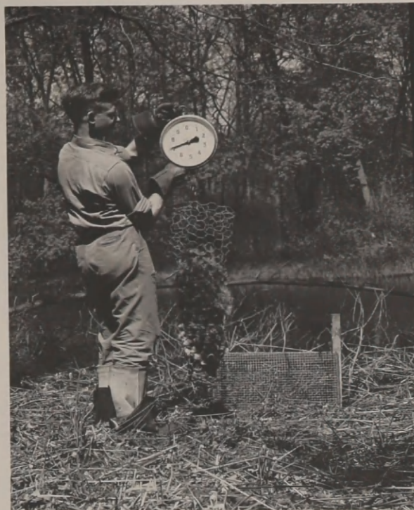
Fig. 14. Dialed scales were used for weighing which had a capacity of 30 lbs. with three revolutions of the pointer. This animal weighed 17 lbs., 1 oz.
