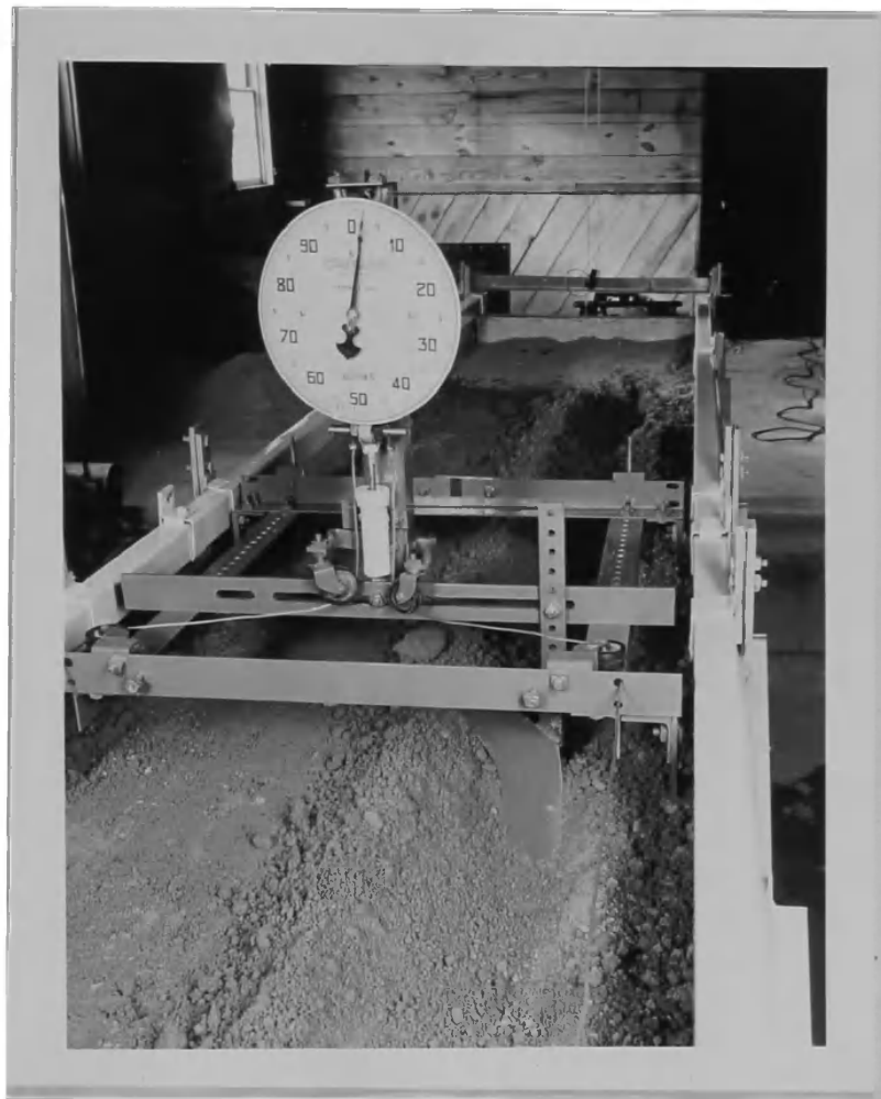
Fig. 13. Soil box, the moving section.
