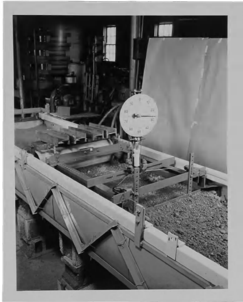
Fig. 12. Soil box, grading and packing.
