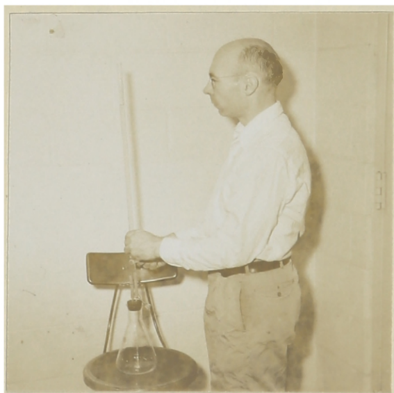
Figure 15. Adding 30 milliliters of \text{Ba}(\text{OH})_2 to the sample.
