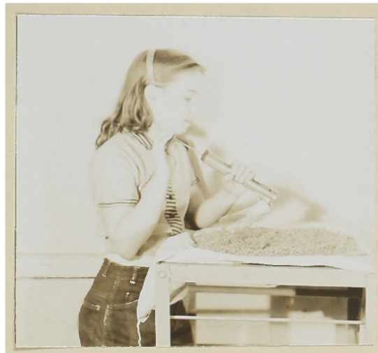
Figure 10. Spraying wheat with distilled water to condition it to the proper moisture level.
