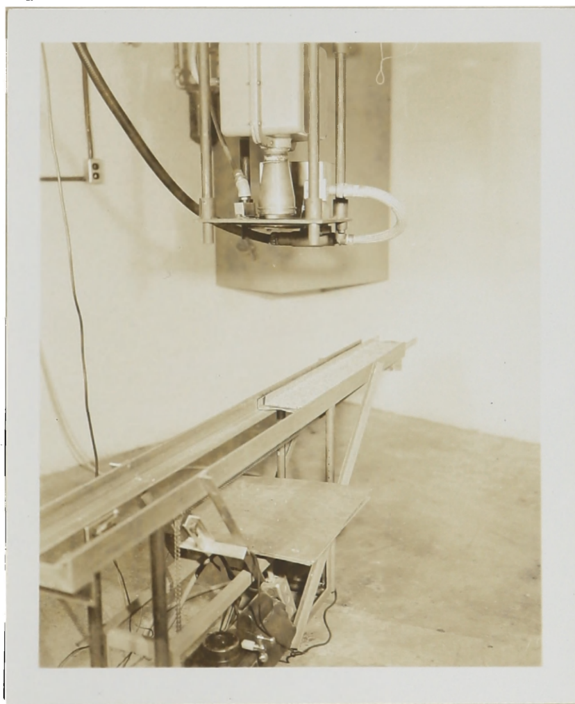
Figure 11. The wheat sample on the conveyor ready to be irradiated.
