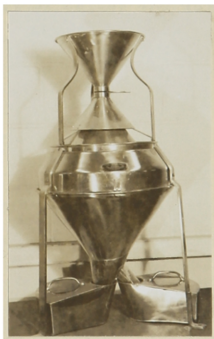
Figure 8. A Boerner Divider which was used to make an equal and random division.
