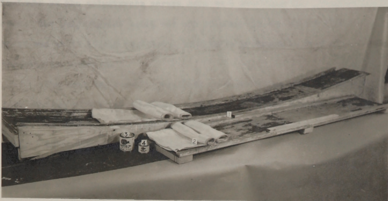
Figure 6. Materials used in laminating with epoxy resin. (1) female mold, (2) glass cloth, (3) modified epoxy resin, (4) resin hardener.
