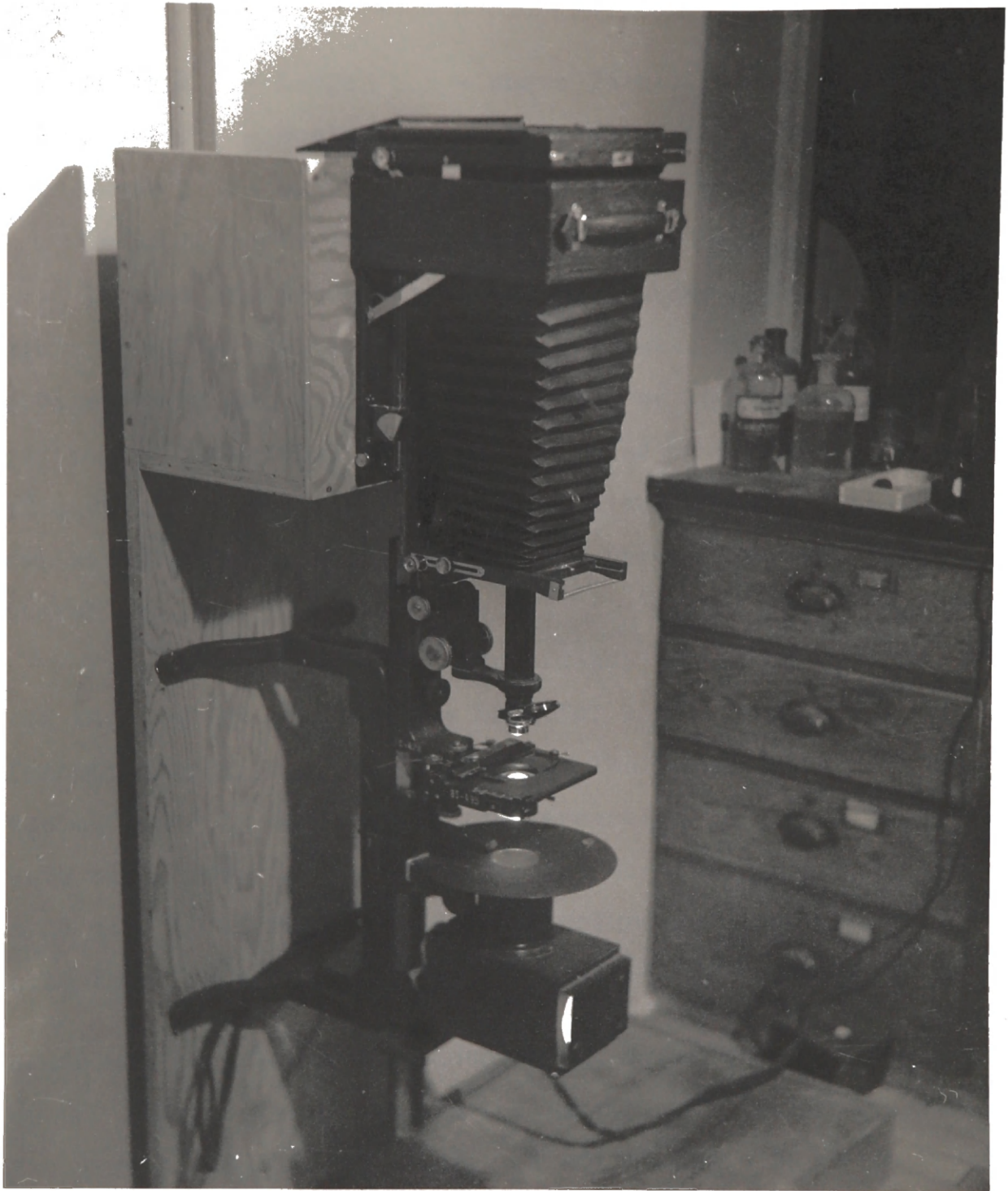
Figure 3. Projection microscope in vertical position with camera fitted on the top.
