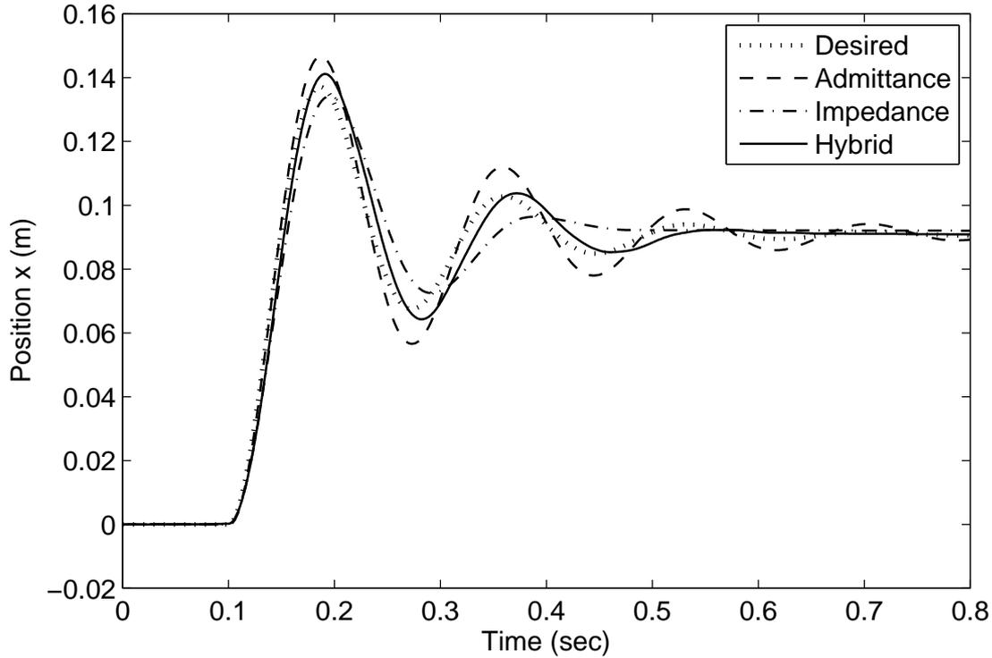
Figure 2.11: Stiff contact position response for  $\delta = 50 \text{ ms}$  and  $n = 0.5$
