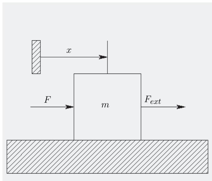
Figure 2.1: A single degree-of-freedom mass interacting with the environment
