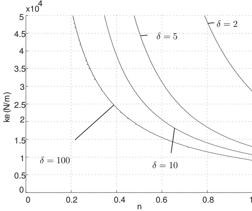
Figure 2.3: Stability boundaries for hybrid impedance and admittance control for different values of  $\delta$
