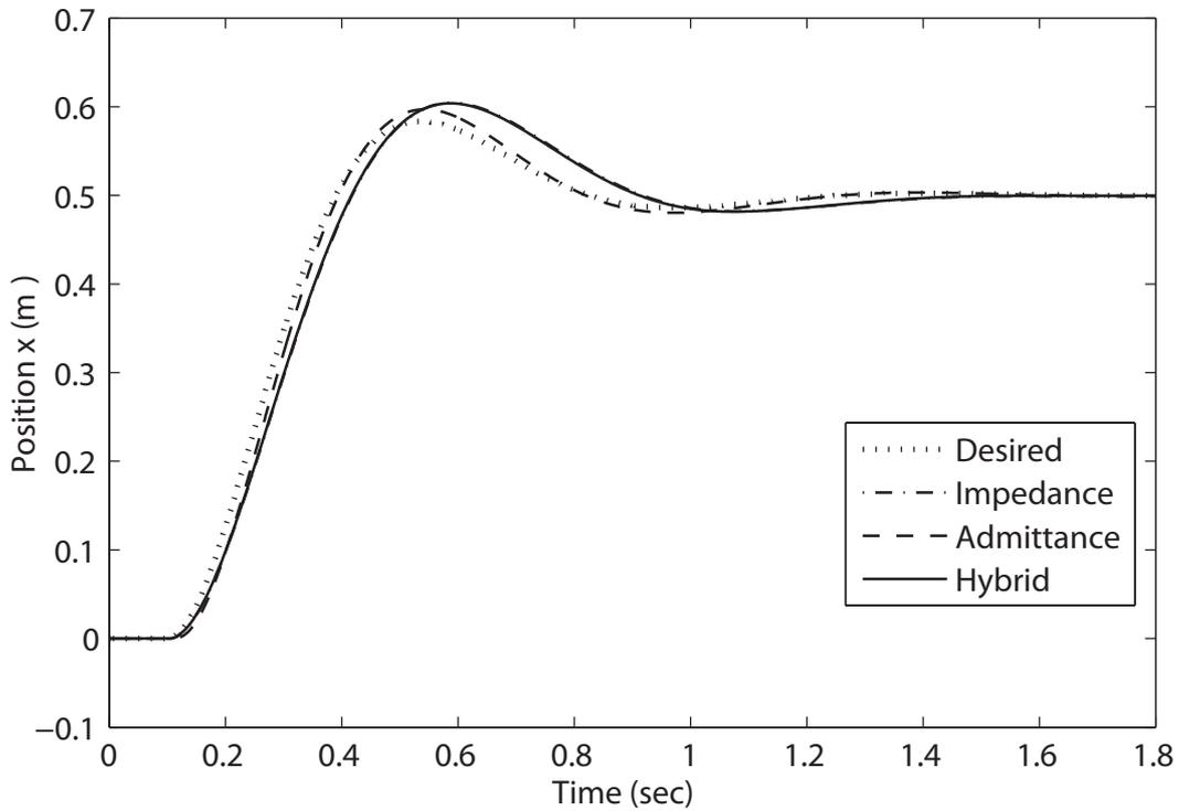
Figure 5.3: Soft contact position response for  $\delta = 50 \text{ ms}$  and  $n = 0.1$
