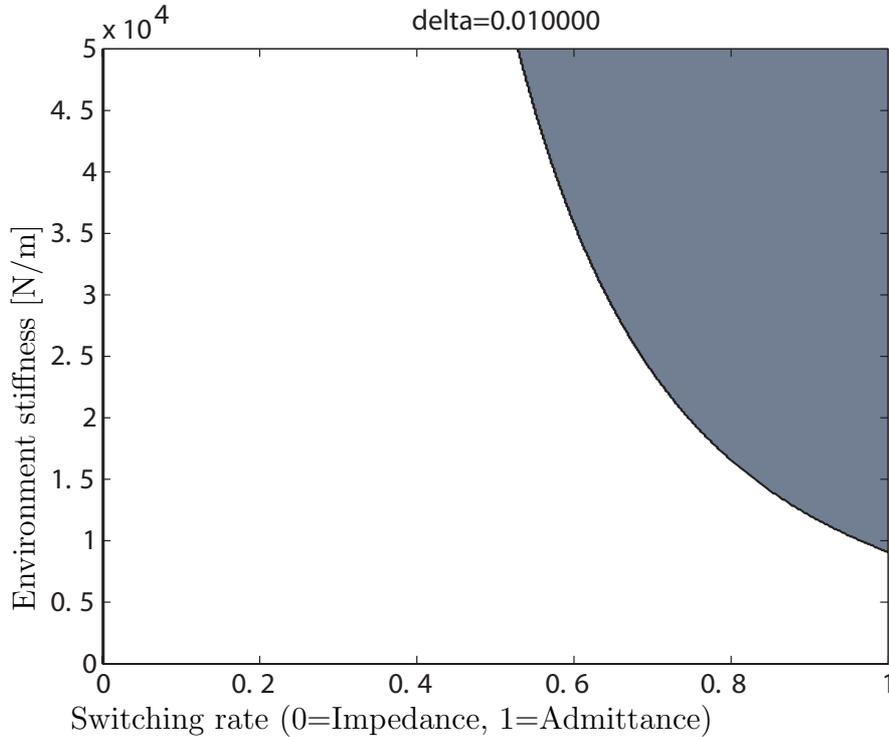
Figure 3.2: Stability boundaries for hybrid impedance and admittance control for  $\delta = 10 \text{ ms}$  and  $K_p = 10000 \text{ N/m}$
