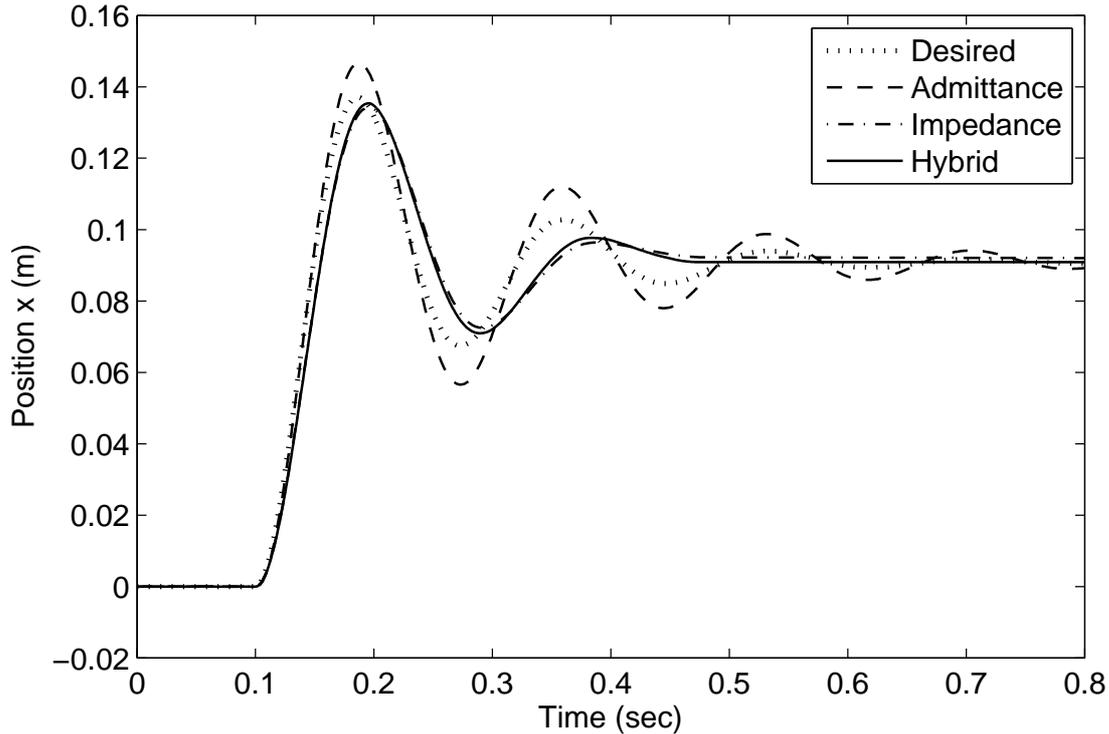
Figure 2.10: Stiff contact position response for  $\delta = 50 \text{ ms}$  and  $n = 0.1$
