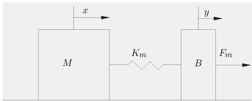
Figure 5.1: Single degree-of-freedom flexible joint model
