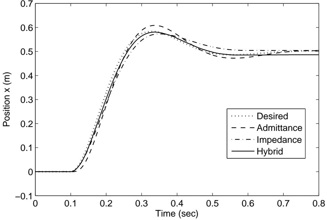
Figure 3.5: Soft contact position response for  $K_p = 10000 \text{ N/m}$ ,  $\delta = 50 \text{ ms}$ , and  $n = 0.5$
