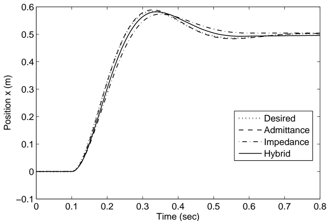
Figure 2.7: Soft contact position response for  $\delta = 50 \text{ ms}$  and  $n = 0.5$
