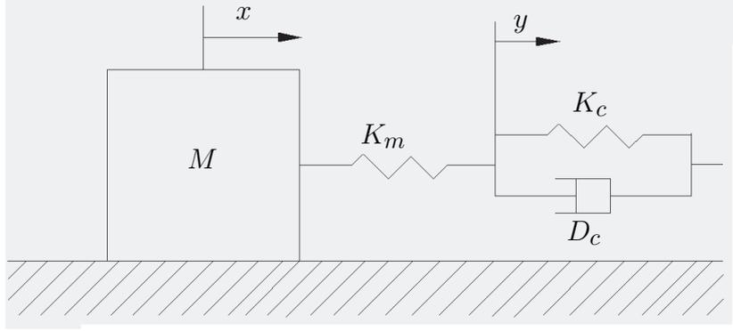
Figure 5.2: Single degree-of-freedom passive impedance for flexible joint model
