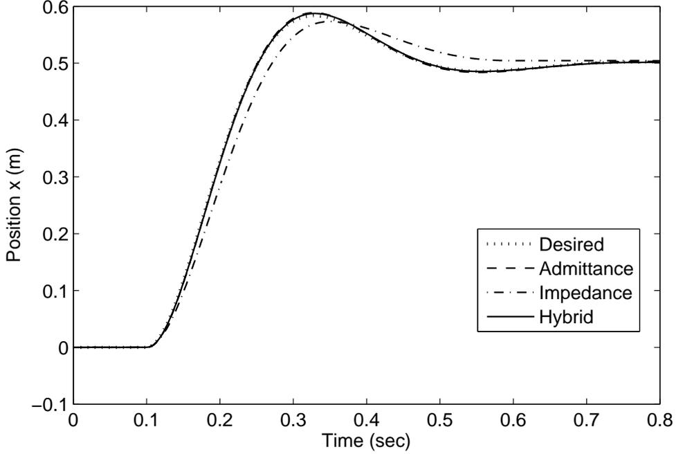
Figure 2.5: Soft Contact position response for  $\delta = 50 \text{ ms}$  and  $n = 0.9$
