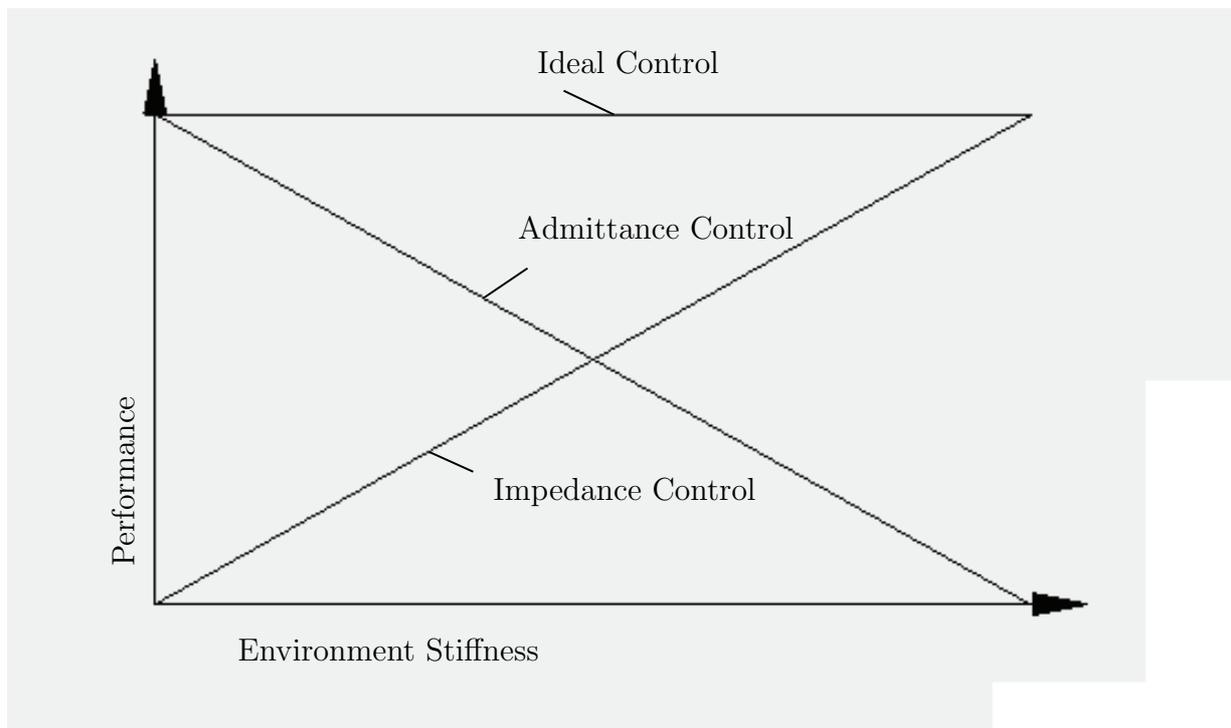
Figure 2.2: Qualitative illustration of the performance of impedance control and admittance control for different environment stiffness
