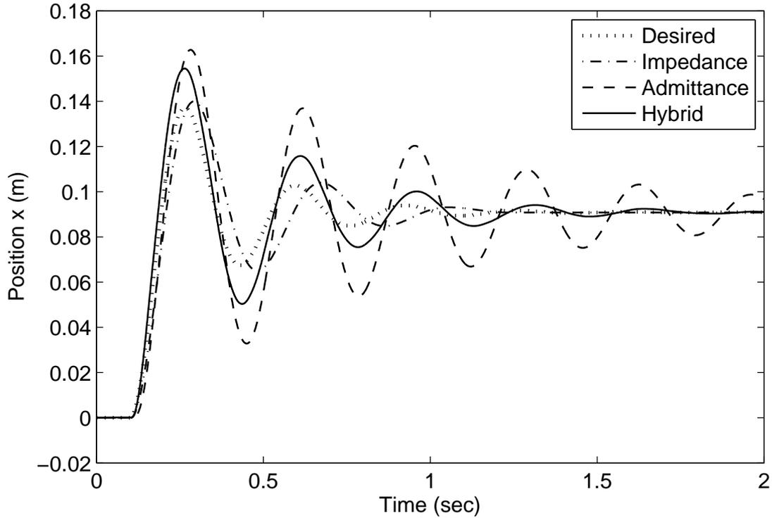
Figure 5.8: Stiff contact position response for  $\delta = 50 \text{ ms}$  and  $n = 0.9$
