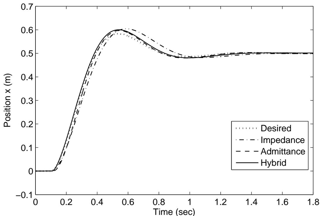
Figure 5.5: Soft contact position response for  $\delta = 50 \text{ ms}$ , and  $n = 0.9$
