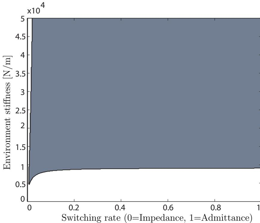
Figure 3.1: Stability boundaries for convex combination of impedance and admittance control
