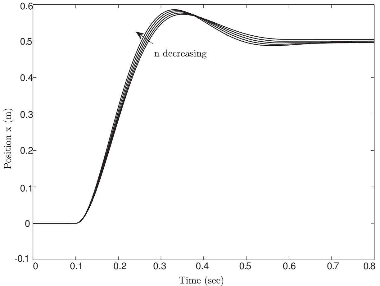
Figure 2.8: Soft Contact position response for  $\delta = 50 \text{ ms}$  and a range of  $n$  values
