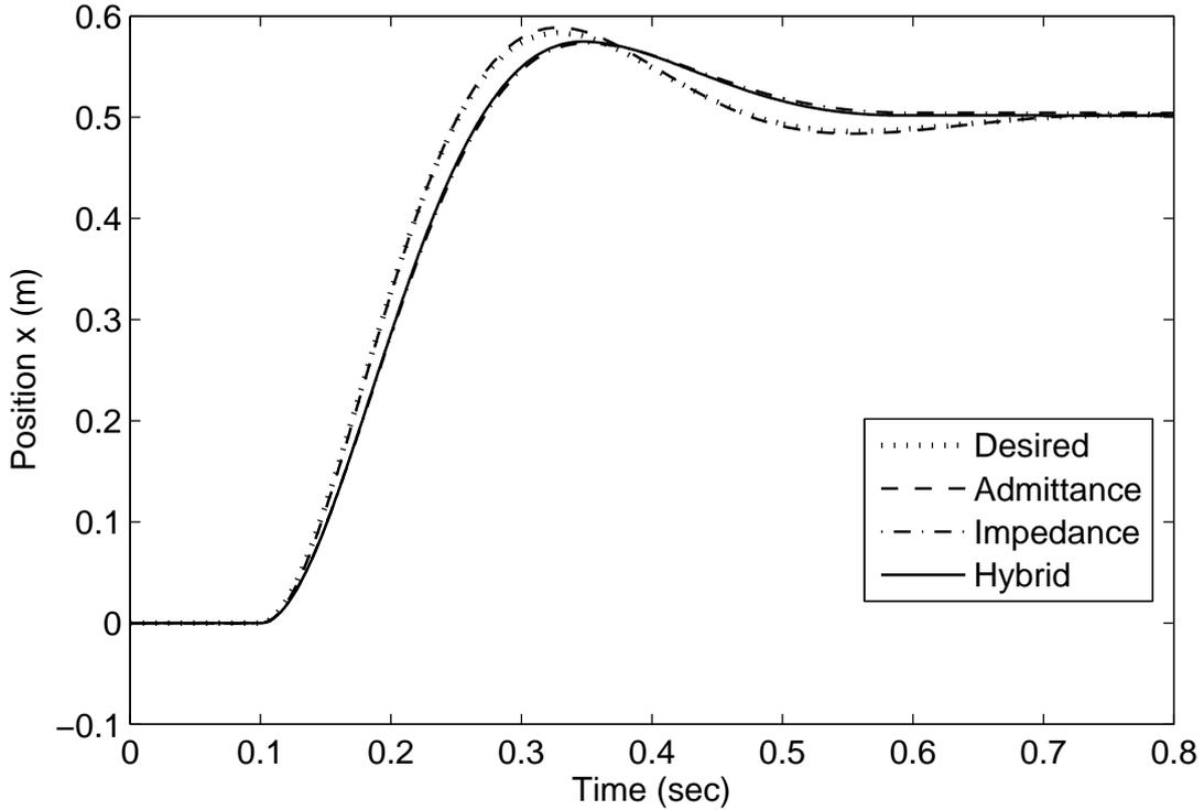
Figure 2.6: Soft contact position response for  $\delta = 50$  ms and  $n = 0.1$
