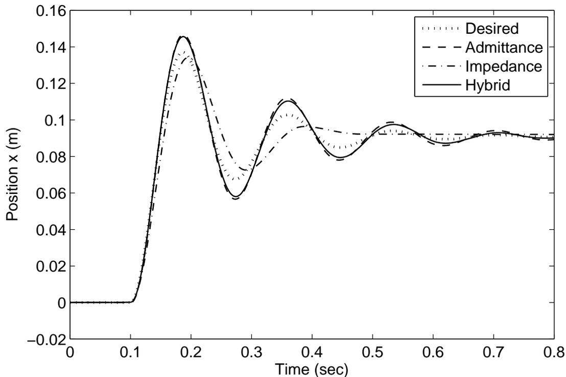
Figure 2.9: Stiff contact position response for  $\delta = 50 \text{ ms}$  and  $n = 0.9$
