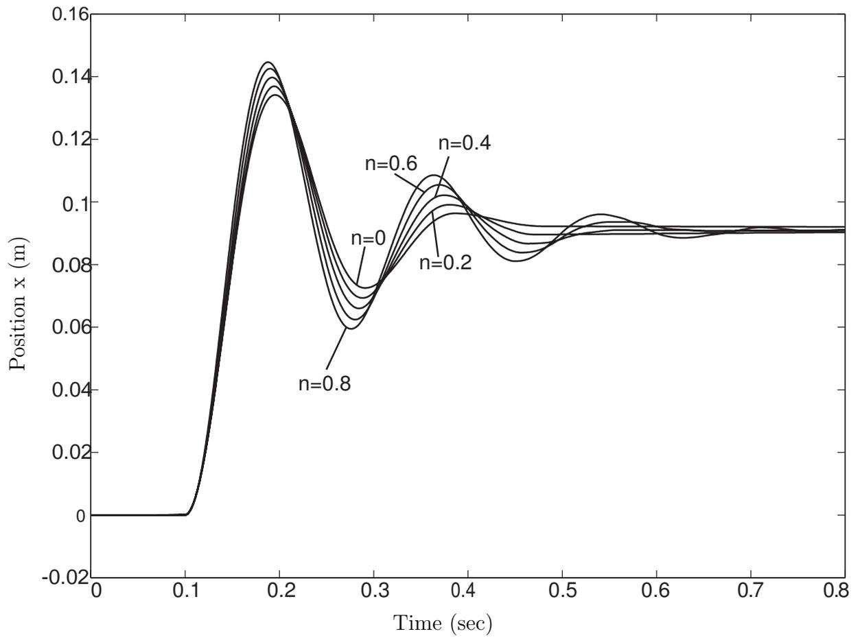
Figure 2.12: Stiff contact position response for  $\delta = 50$  ms and a range of  $n$  values
