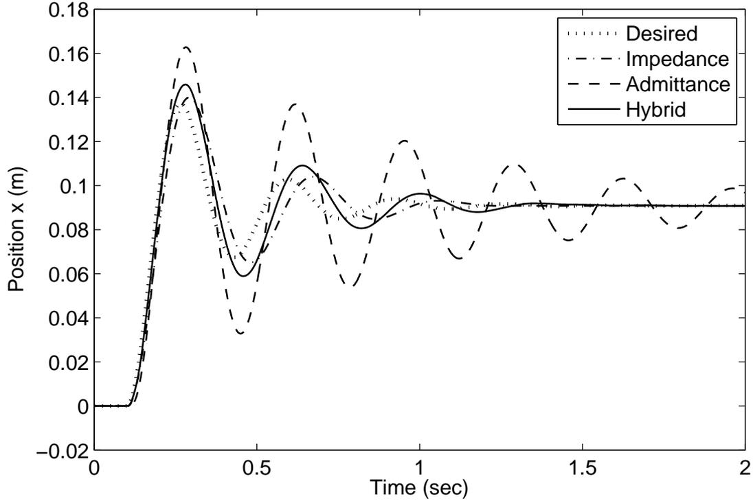
Figure 5.7: Stiff contact position response for  $\delta = 50 \text{ ms}$  and  $n = 0.5$
