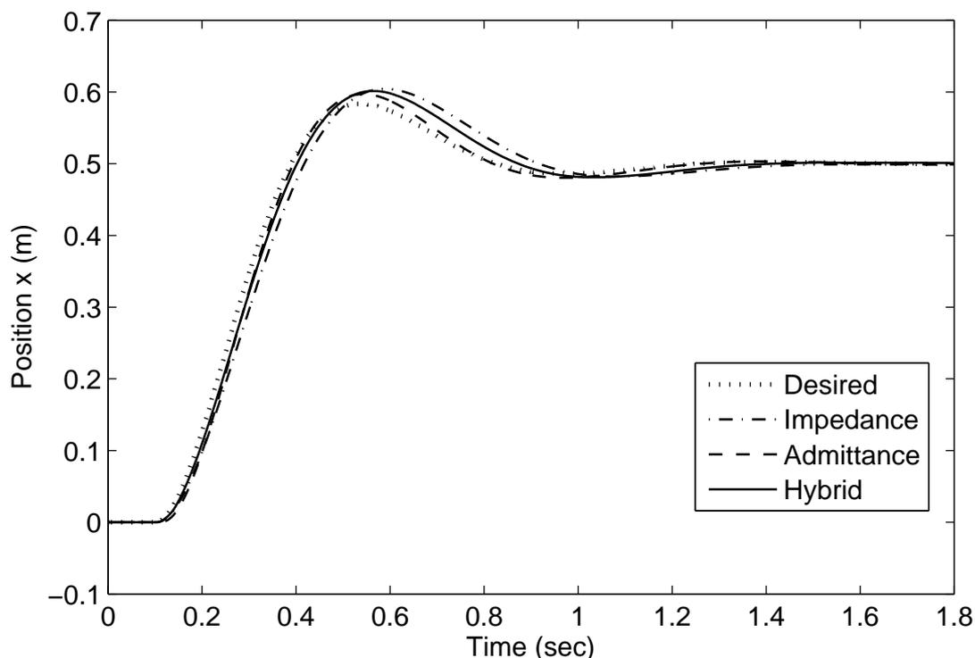
Figure 5.4: Soft contact position response for  $\delta = 50$  ms and  $n = 0.5$
