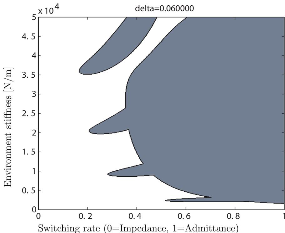
Figure 3.3: Stability boundaries for hybrid impedance and admittance control for  $\delta = 60 \text{ ms}$  and  $K_p = 10000 \text{ N/m}$
