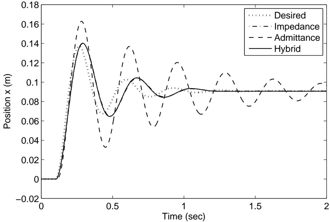
Figure 5.6: Stiff contact position response for  $\delta = 50 \text{ ms}$  and  $n = 0.1$
