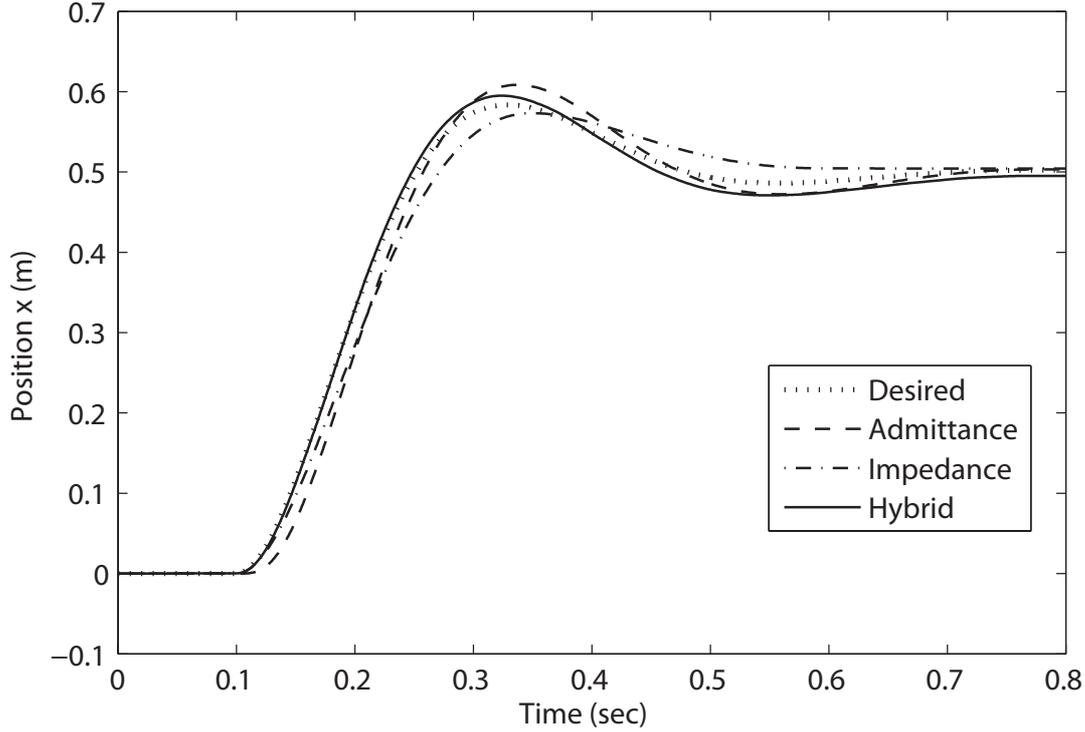
Figure 3.4: Soft contact position response for  $K_p = 10000 \text{ N/m}$ ,  $\delta = 50 \text{ ms}$ , and  $n = 0.9$
