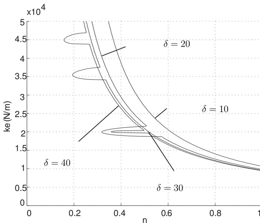
Figure 2.4: Stability boundaries for hybrid impedance and admittance control for  $\delta$  values 10 *ms*, 20 *ms*, 30 *ms*, and 40 *ms*
