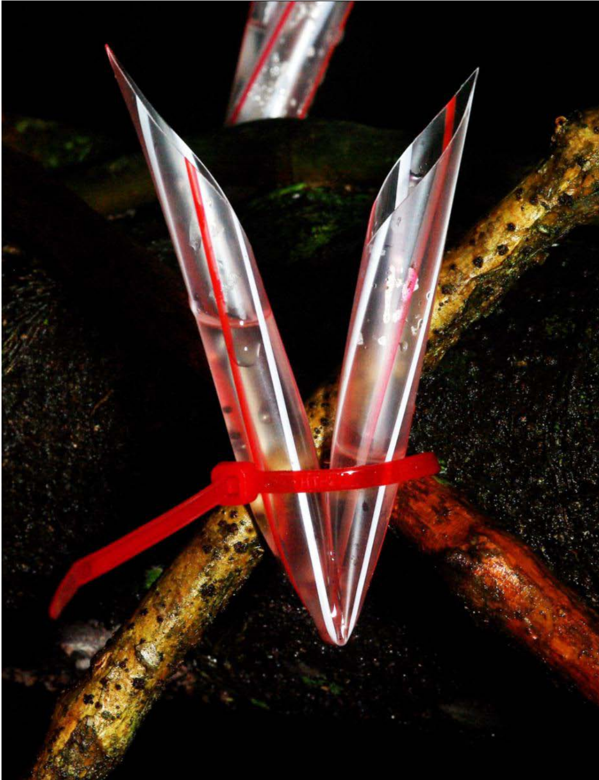
Figure 4.3: Straws were cut to create a tip that would aid in capturing rain water. Straws were attached to woody vegetation using zip-ties and fence staples taking care not to crush the straw.
