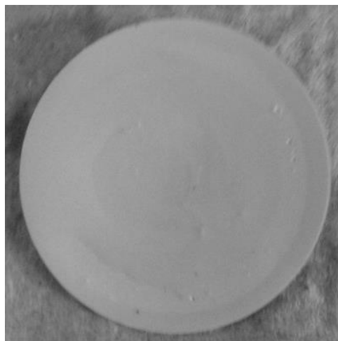
Figure 3.11: PP coated PVDF membrane (feed surface) after DCMD of whey solution.
