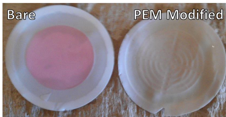
Figure 4.14: Comparison of irreversible membrane staining from uncharged, hydrophobic oil-soluble dye for bare and PEM modified membranes after oil emulsion cross-flow filtration at 80 mL/min and an applied transmembrane pressure of 2 bar.
