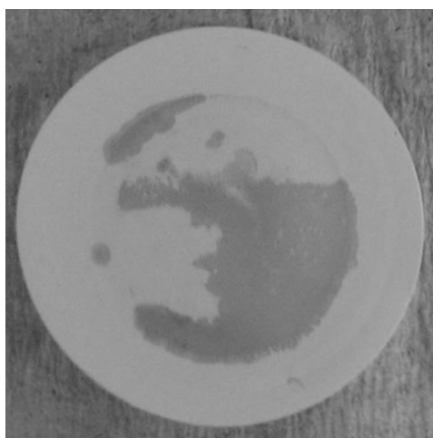
Figure 3.9: Untreated PVDF membrane (feed surface) after DCMD of whey solution.
