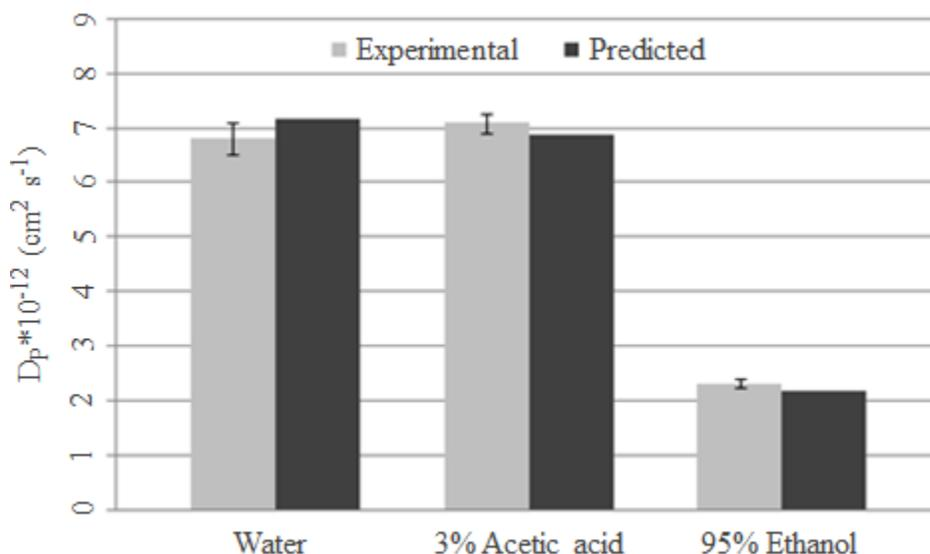
**Figure 4.3** Mean ( $\pm$ SD, N=3) experimental and predicted diffusion coefficients of BPA in LDPE contacting with three different food simulants.
