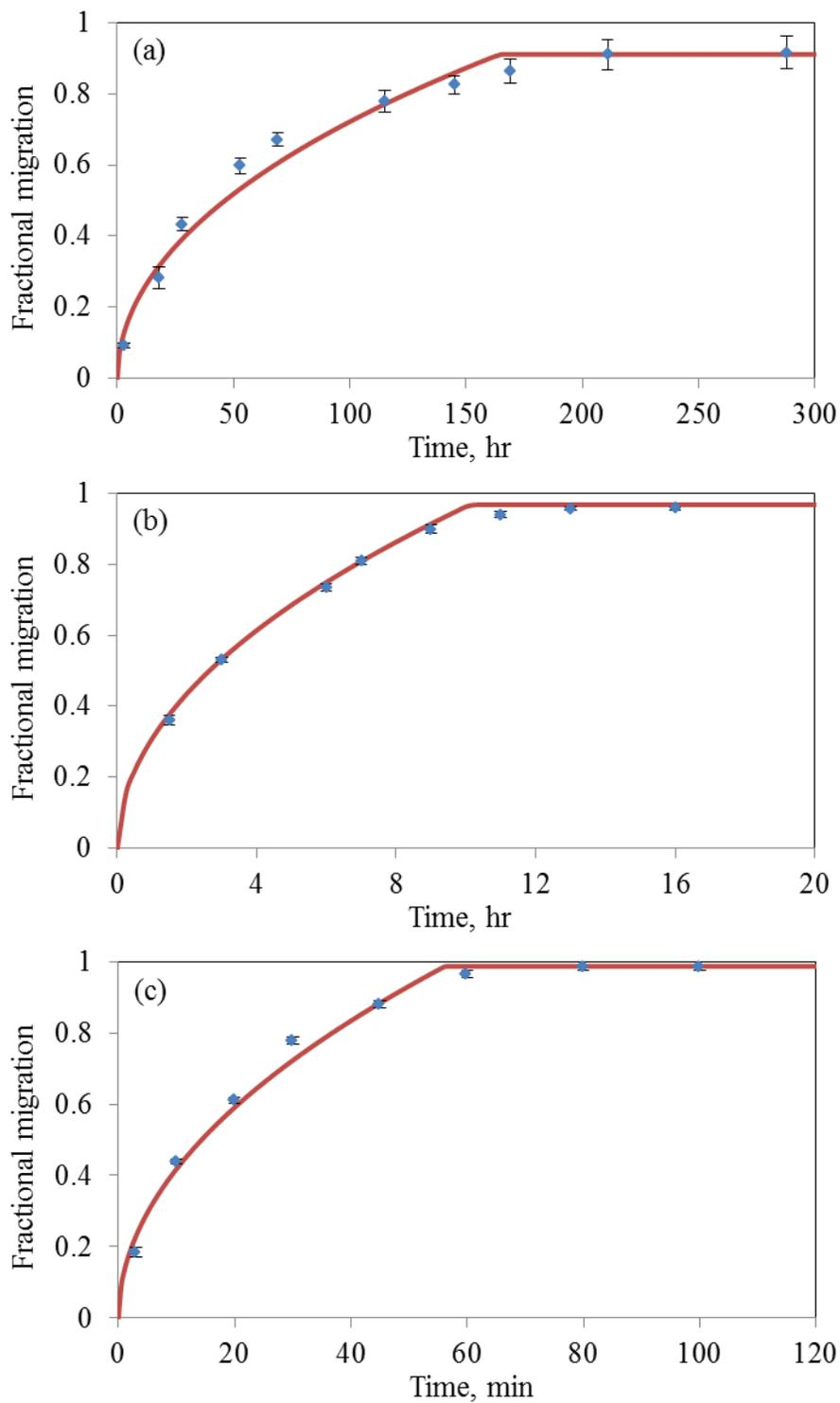
**Figure B6** Amount of BPA migrated from LDPE into water at (a) 40 °C, (b) 60 °C and (c) 80 °C relative to the initial amount in the polymer ( $2.66 \text{ mg g}^{-1}$ ).
