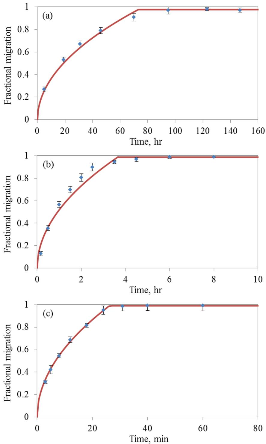
**Figure B2** Amount of BPA migrated from LDPE into 3% acetic acid at (a) 40 °C, (b) 60 °C and (c) 80 °C relative to the initial amount in the polymer ( $1.42 \text{ mg g}^{-1}$ ).
