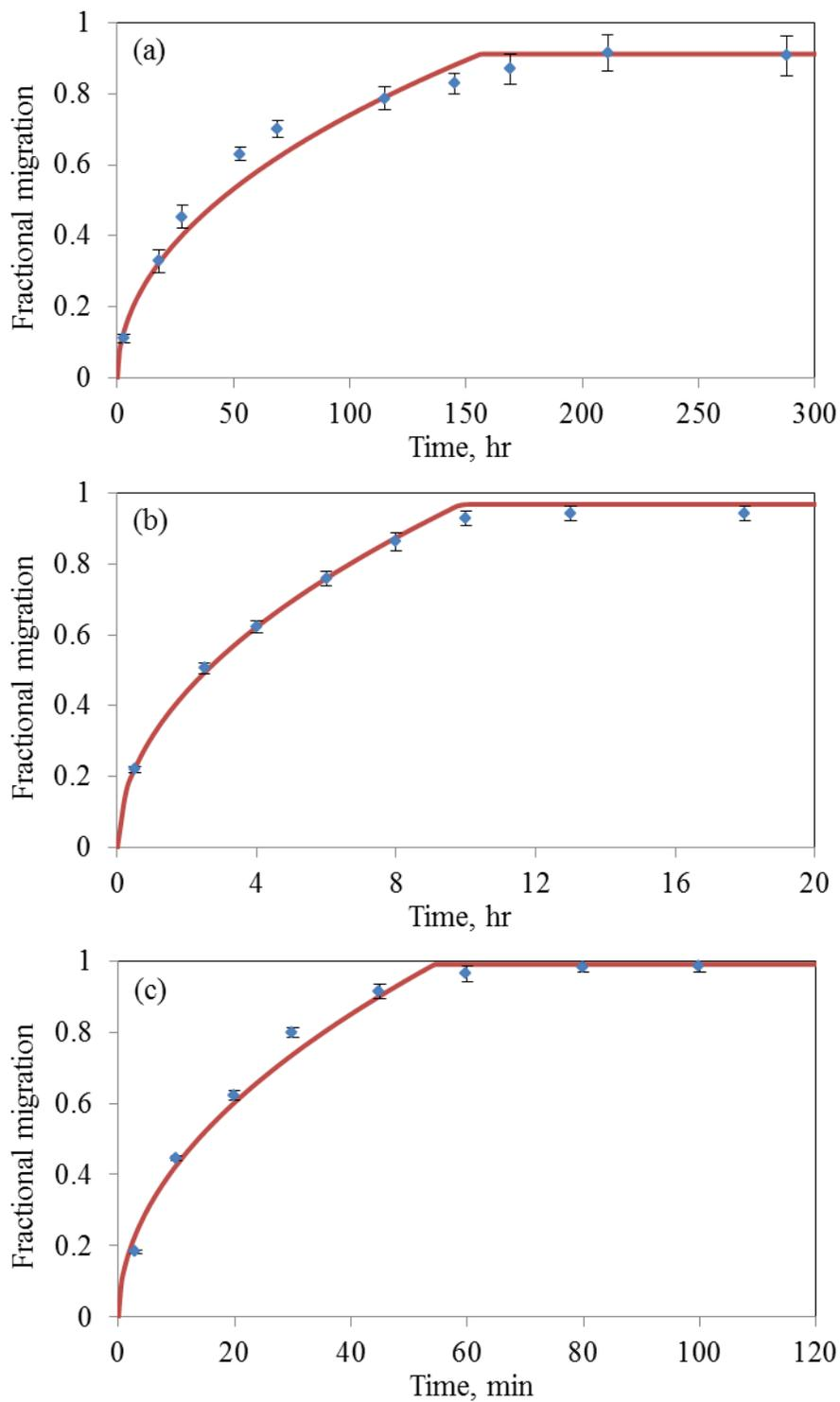
**Figure B7** Amount of BPA migrated from LDPE into 3% acetic acid at (a) 40 °C, (b) 60 °C and (c) 80 °C relative to the initial amount in the polymer ( $2.66 \text{ mg g}^{-1}$ ).
