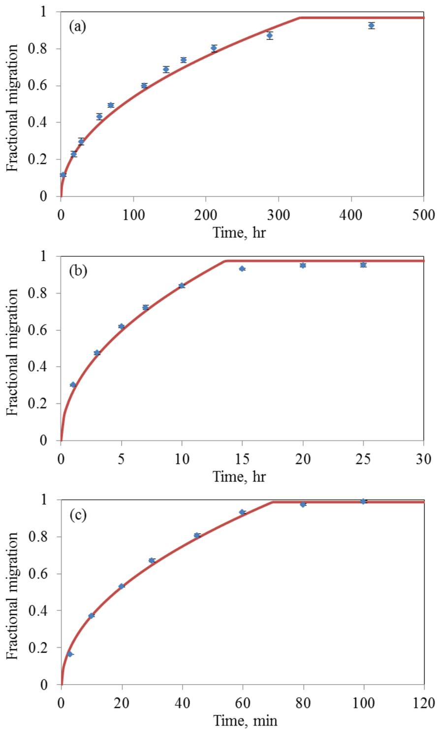
**Figure B8** Amount of BPA migrated from LDPE into 95% ethanol at (a) 40 °C, (b) 60 °C and (c) 80 °C relative to the initial amount in the polymer ( $2.66 \text{ mg g}^{-1}$ ).
