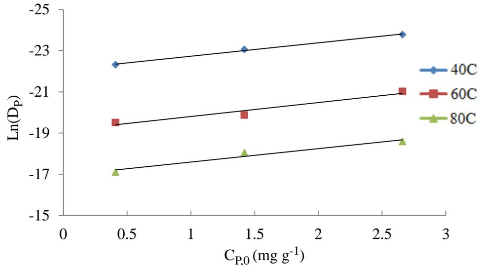
**Figure 4.4** Diffusion coefficient of BPA in LDPE in contact with water as a function of initial BPA concentration at different temperatures.
