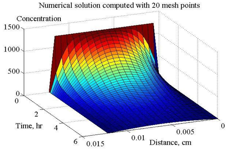
**Figure 4.5** Concentration profiles (2D and 3D) of BPA in LDPE contact with water at 60 °C with an initial BPA concentration of  $1.42 \text{ mg g}^{-1}$ .
