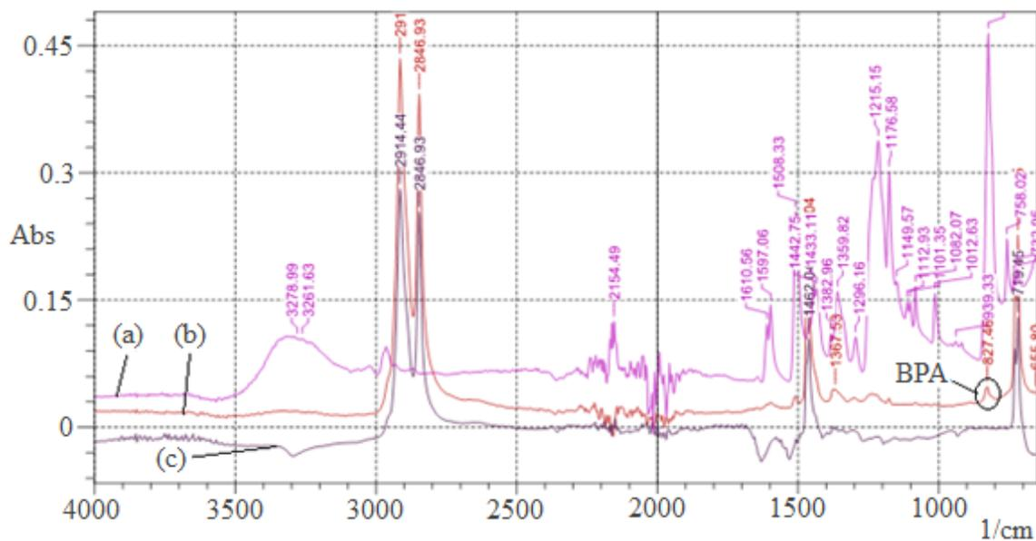
**Figure A1** FTIR graph of (a) BPA, (b) LDPE + BPA (0.5 wt%) and (c) LDPE.
