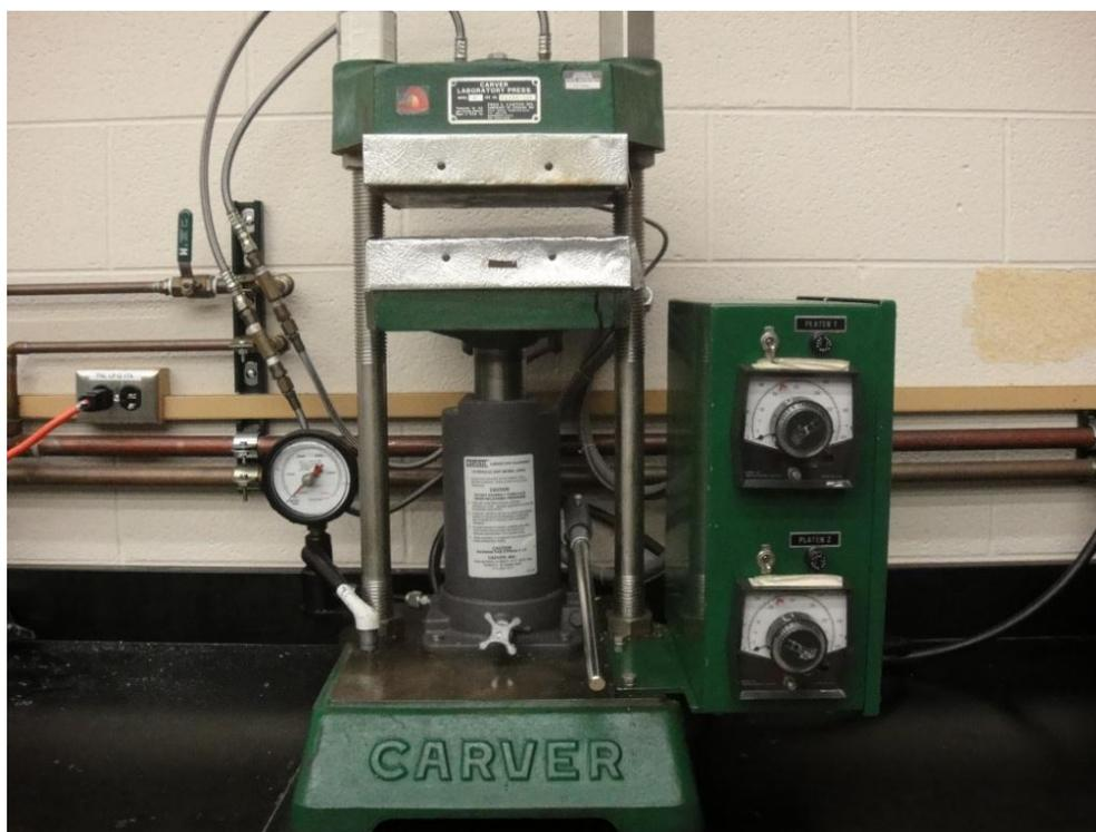
**Figure 3.3** Carver Laboratory Press used for compression molding.
