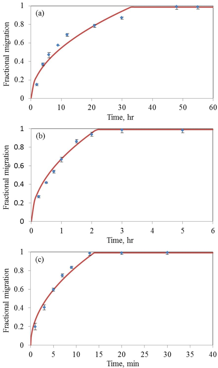
**Figure B4** Amount of BPA migrated from LDPE into 3% acetic acid at (a) 40 °C, (b) 60 °C and (c) 80 °C relative to the initial amount in the polymer ( $0.41 \text{ mg g}^{-1}$ ).
