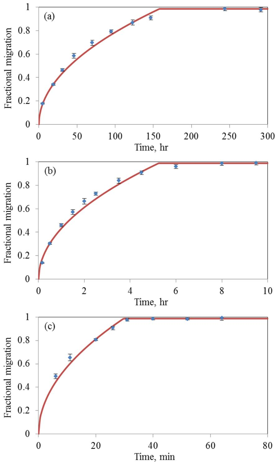
**Figure 4.2** Amount of BPA migrated from LDPE into 95% ethanol at (a) 40 °C, (b) 60 °C and (c) 80 °C relative to the initial amount in the polymer ( $1.42 \text{ mg g}^{-1}$ ).
