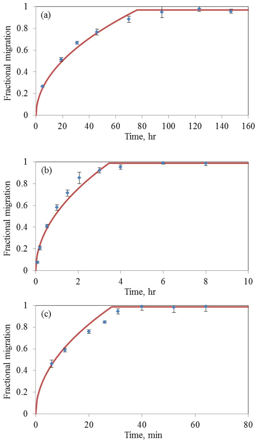
**Figure B1** Amount of BPA migrated from LDPE into water at (a) 40 °C, (b) 60 °C and (c)
