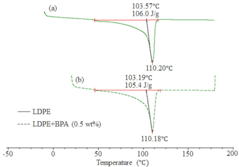
**Figure A2** DSC graph for (a) LDPE and (b) LDPE + BPA (0.5 wt%).
