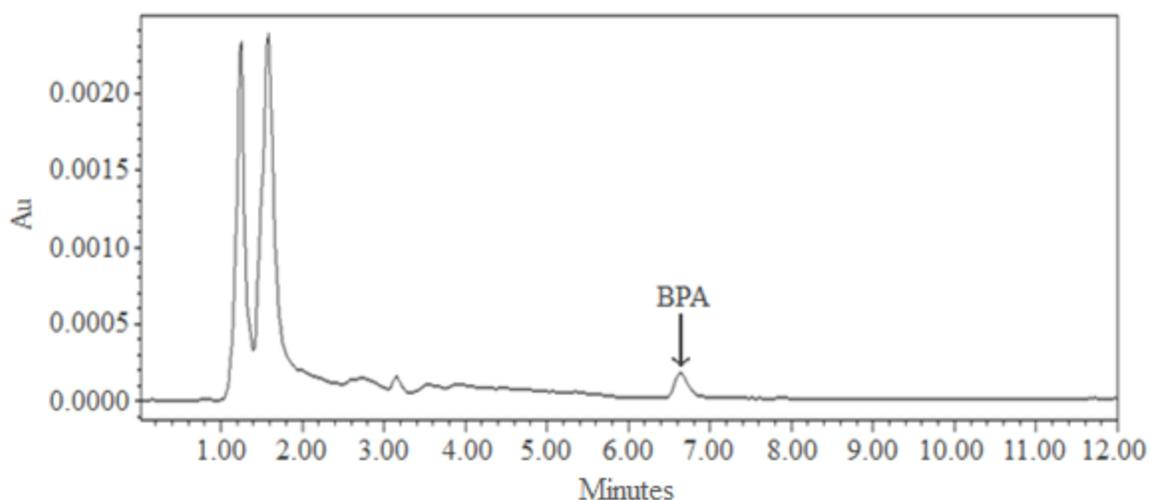
**Figure 4.1** HPLC-UV chromatogram of a standard solution containing  $10\ \mu\text{g L}^{-1}$  BPA.
