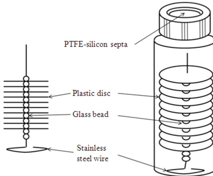
**Figure 3.4** Apparatus for two-sided contact migration testing.
