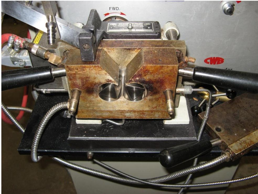
**Figure 3.2** Electrically heated three-piece mixer with two roller style mixing blades.
