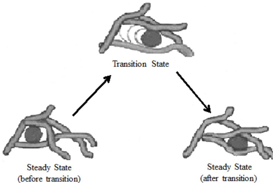
**Figure 2.2** Diffusion process of a small molecule in the polymer matrix.
