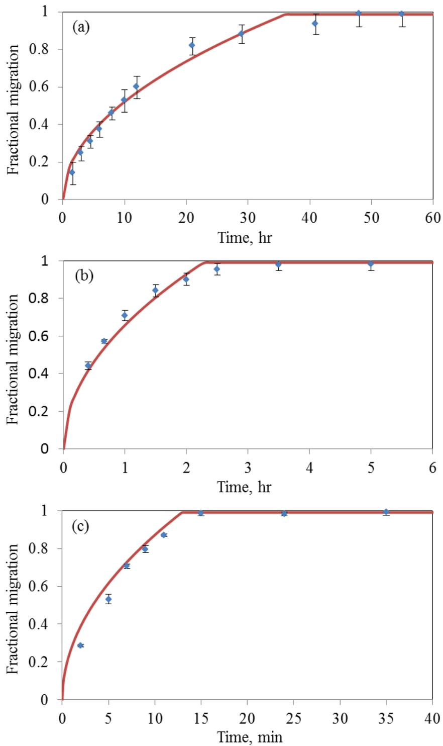
**Figure B3** Amount of BPA migrated from LDPE into water at (a) 40 °C, (b) 60 °C and (c) 80 °C relative to the initial amount in the polymer ( $0.41 \text{ mg g}^{-1}$ ).
