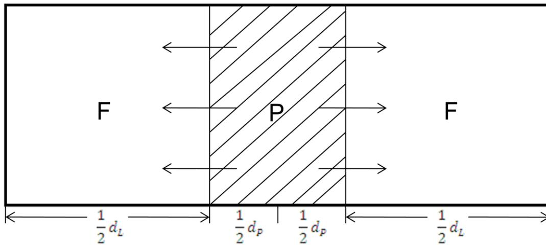
**Figure 2.3** Two-sided contact migration between the polymer (P) and food simulant (F).
