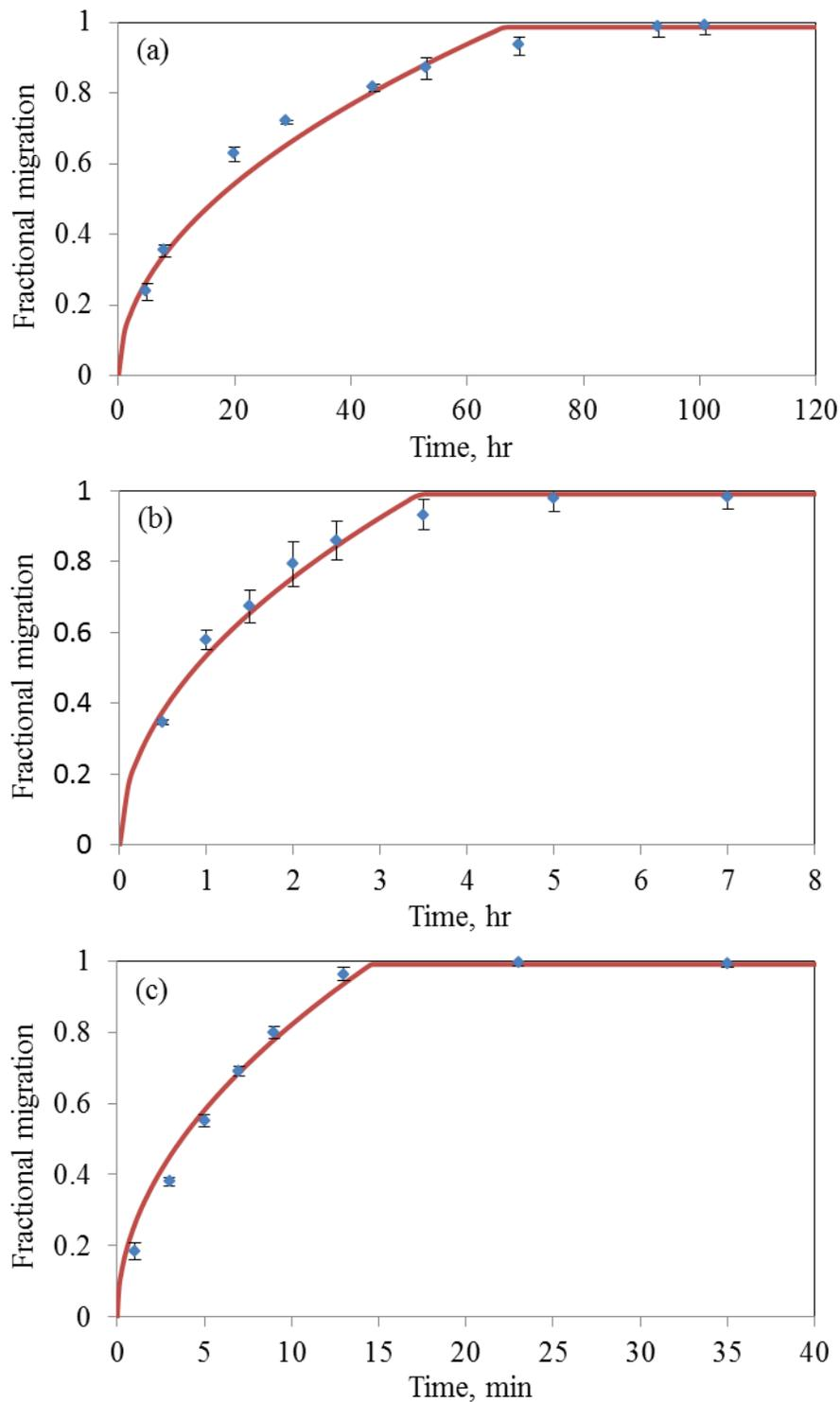
**Figure B5** Amount of BPA migrated from LDPE into 95% ethanol at (a) 40 °C, (b) 60 °C and (c) 80 °C relative to the initial amount in the polymer ( $0.41 \text{ mg g}^{-1}$ ).
