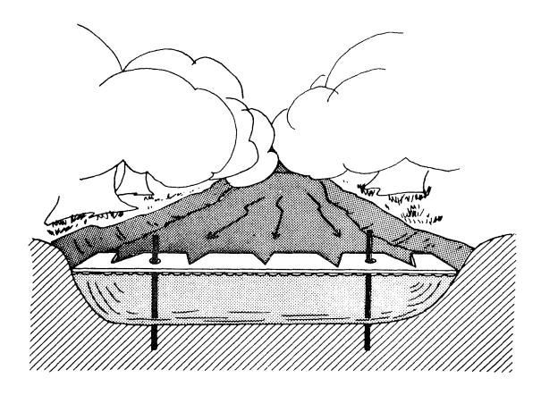
Figure 3. Schematic diagram of device used to collect floating pupal exuvia in Augusta Creek, and in the artificial stream system.
