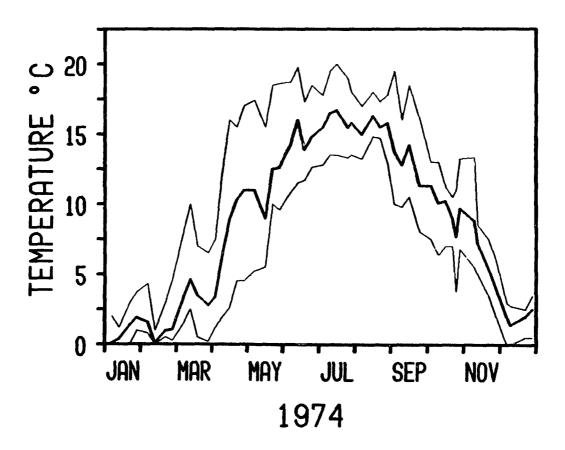
Figure 2. Annual temperature pattern for Augusta Creek, site B, 1974. Given are mean daily and weekly minimum and maximum temperatures.
