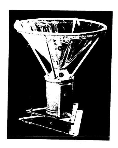
Figure 1.1. Sequential rain sampler. A, funnel; B, cover; C, platform with three leveling bolts; and D, collar.
