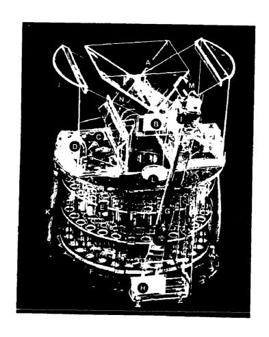
Figure 1.2. Mechanism for the sequential rain sampler. A, tipping bucket; B, bucket bearing; C, drain; D, plexiglass box and siphon; E, collection tube rack and tubes; F, turntable; G, pivoting arm; H, advancing block; I, electronic switch; J, stationary stop piece; K, drain tube; L, level; M, plexiglass arm; and N, counterweights.
