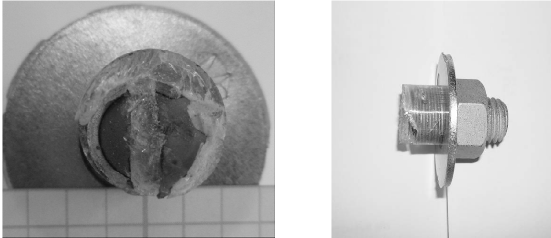
Figure 1.10: Injection bolt failure with 3.18 mm wall thickness insert.
