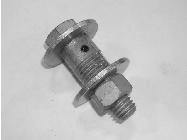
Figure 1.9 – Bolt assembly and injected insert pre-loaded to 2.82 N-m.
