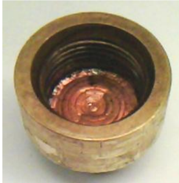
Figure 6. The seal adapter contains a thin copper membrane.
