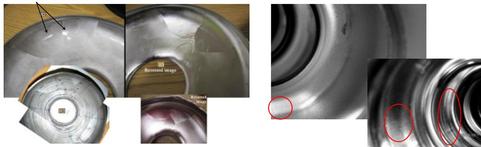
Figure 1.3: Surface defects in a well prepared SRF cavity cell.
