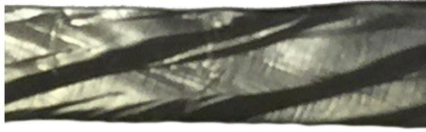
Figure 2.10: Surface topography of deformed single crystal Nb [12]
